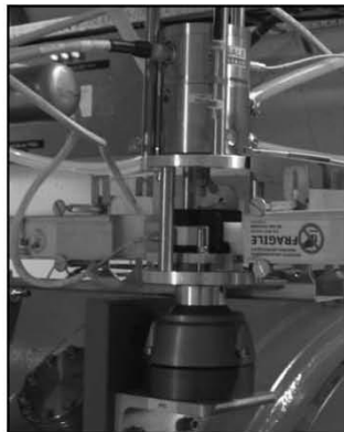
2 Hydrostatic levelling system sensor in LHC environment. Dimensions are: 140 mm height, 100 mm of diameter
