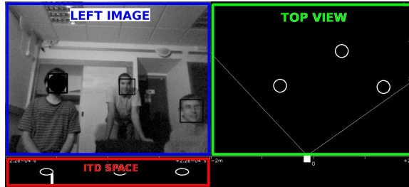
Figure 7.5: Snapshot of the visualization tool. Top-left (blue-framed): The original left image overlaid with one bounding box per detected face. In addition, an intensity-coded circle appears when the face emits a sound. The darker the circle, the higher the speaking probability. Top-right (green-framed): A bird-view of the 3D scene, in which each circle corresponds to a detected head. Bottom-left (red-framed): The ITD space. The projected faces are displayed with an ellipse while extracted ITD values are shown as bars in a histogram.
