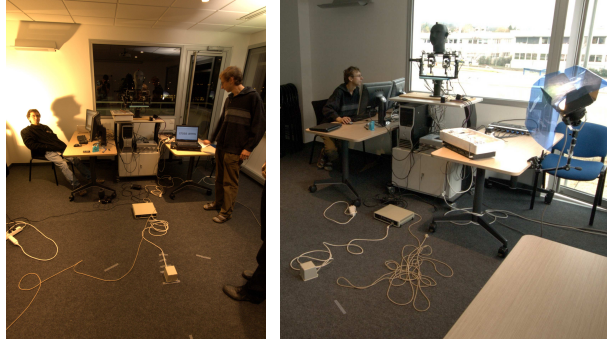
Figure A.3: Two views of the recording environment. The POPEYE robot is in one side of the room. As shown, the sequences were shot with and without daylight providing for lighting variations. Whilst two diffuse lights were included in the setup to provide for good illumination, no devices were used to modify neither the illumination changes nor the sound characteristics of the room. Hence, the recordings are affected by all kind of audio and visual interferences and artifacts present in natural indoor scenes.
