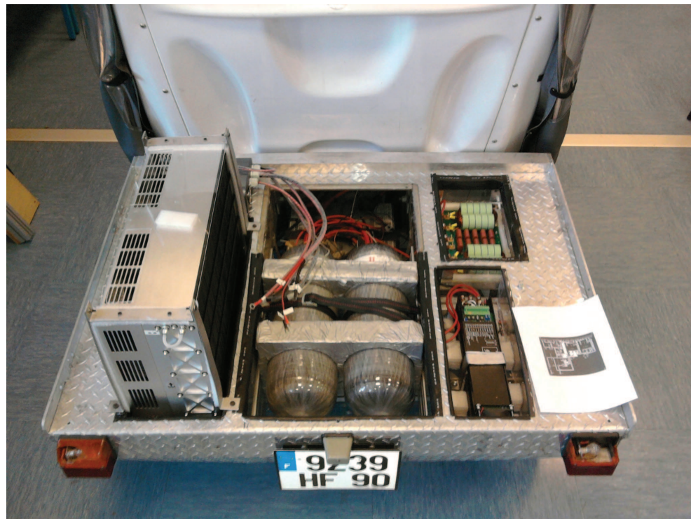
FIGURE 63. SeTcar : Zoom on the fuel cell system
