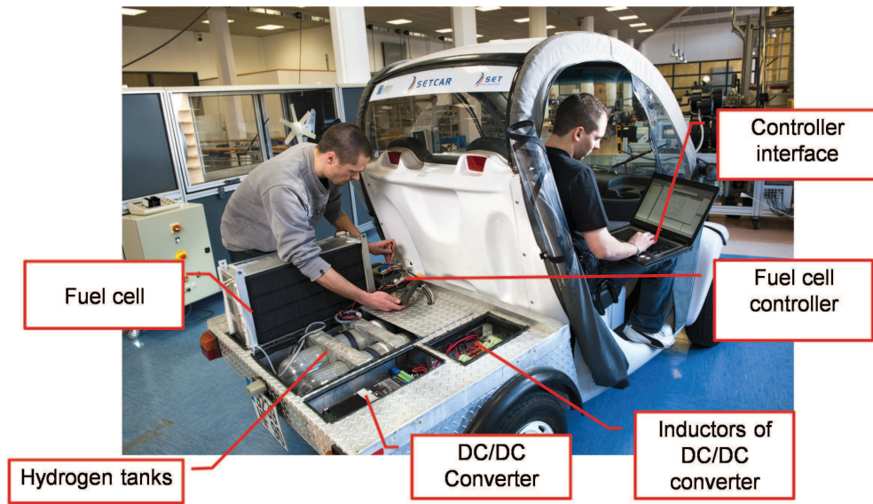
FIGURE 62. SeTcar : hybrid electric vehicle based on a fuel cell as a primary source of energy
