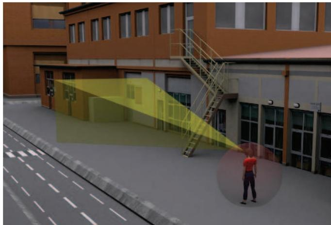
FIGURE C.2 – Example of Pedestrian Frustum, composed of a Spherical Frustum and a Pyramidal Frustum
