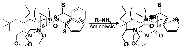
Figure II. 16: PNAM-DT aminolysis with a primary amine.
