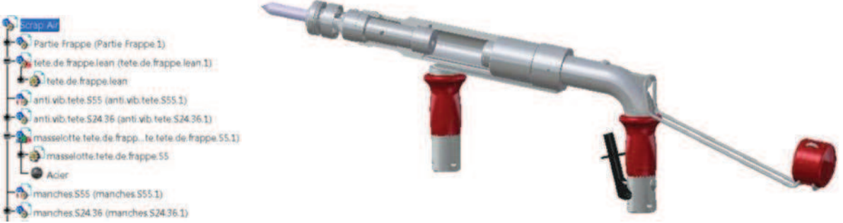
Figure 71. Parametric and skeletal CAD model of a generic pneumatic scraper
