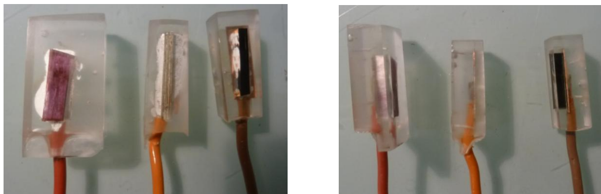
Figure 41: Views of three different electrodes. From left to right: lepidolite, muscovite and biotite.
