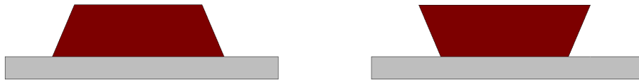
Figure 4.7: Schematic cross-sectional view of positive (left) and negative (right) photoresists after their UV insulation and development. Note the overhang of the negative PR.
