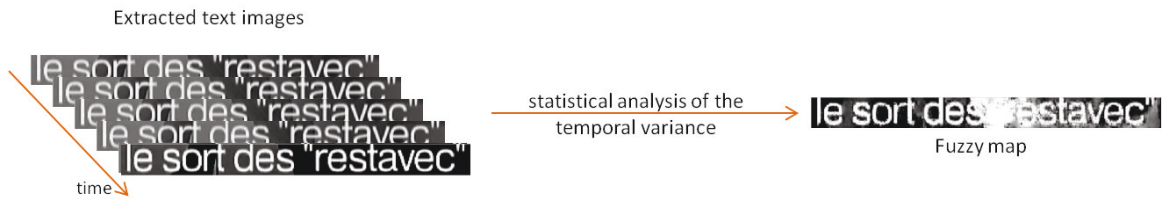
Figure 4.4: Multi-frame integration: obtained fuzzy map; dark pixels are those presenting high variations while bright ones are those with low variations.
