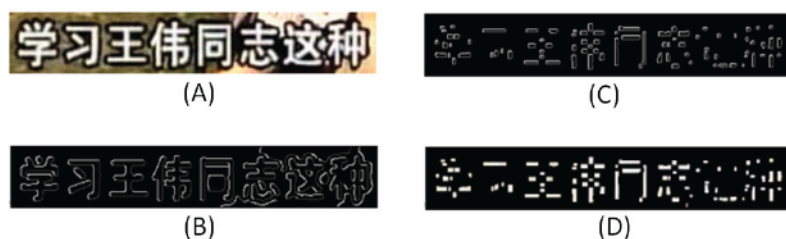
Figure 2.5: Illustration of text pixel selection: (A) original text image, (B) Canny detector result, (C) parallel edge lines and (D) selected text pixels [YGH04].
