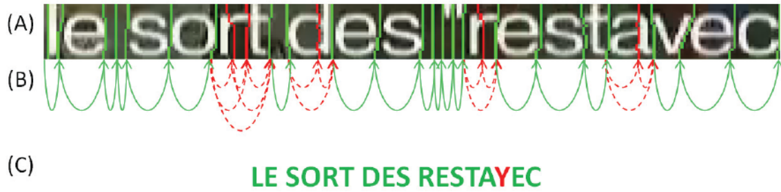
Figure 4.12: An example of recognized text: (A) the segmented text image: green and red separations represent respectively “accurate” and “risky” segmentations, (B) characters candidates: green arcs illustrate characters located between successive “accurate” segmentations and red dotted arcs represent different possible configurations of characters related to “risky” segmentations, and (C) the recognized text.
