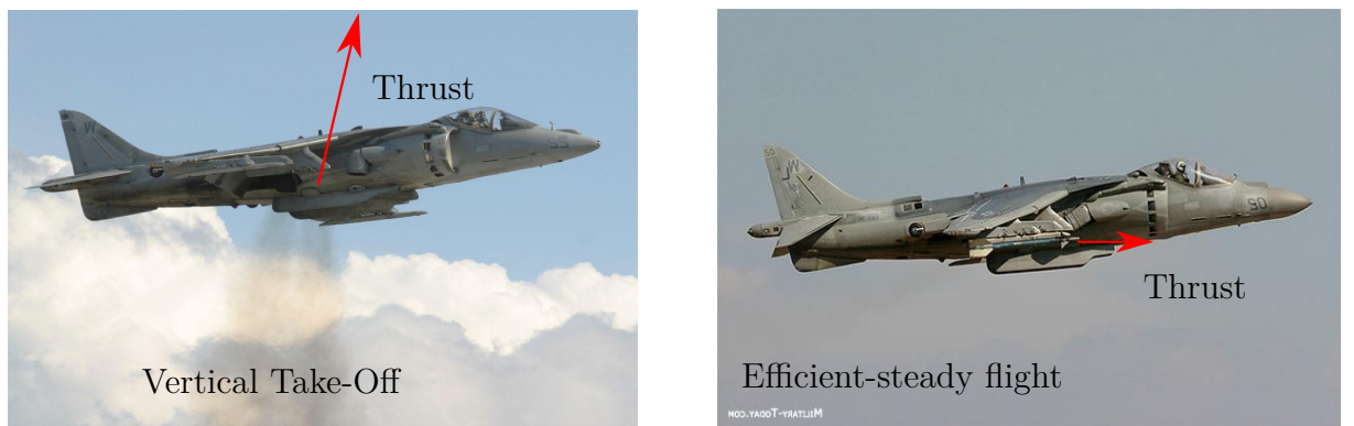
Figure 2.7: A tilting-thrust convertible: AV-8B Harrier II (source Wikipedia ).
