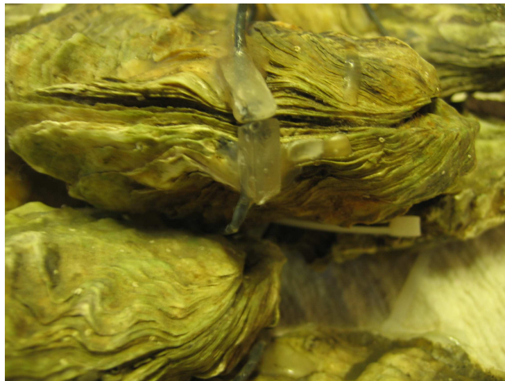
Figure 3.1: Two electrodes stuck on an oyster. Picture taken by the MolluSCAN Eye team.
