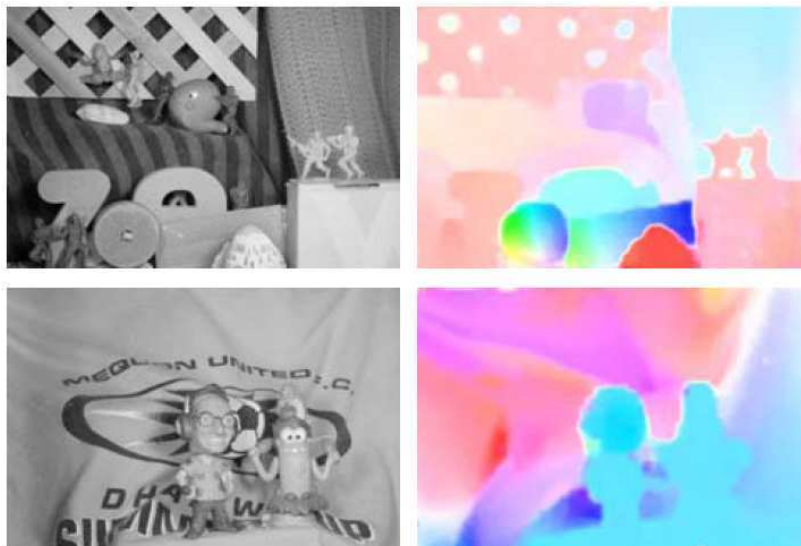
Fig. 13: The 10th frame of the Army sequence (upper row) and Mequon sequence (lower row) and our estimated (color-encoded) optical flow fields.
