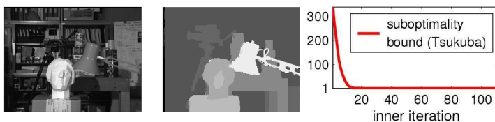
Fig. 2: Online approximation factors computed by FastPD for a benchmark stereo matching problem. Notice how quickly these approximation factors approach the value of 1, meaning that the corresponding estimated solutions are almost optimal.
