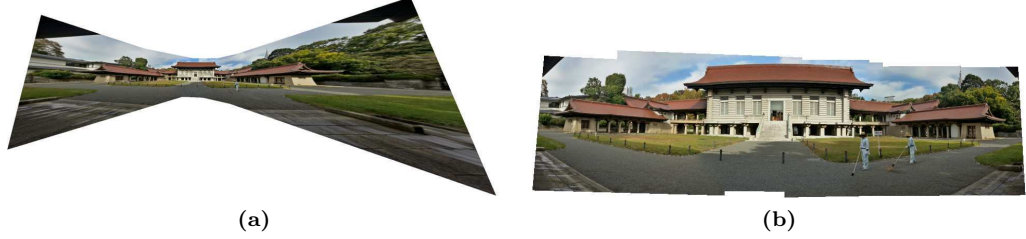
Figure 1.9: Planar vs. spherical coordinates. (a) Map created using the original images and a perspective projection model. The large FOV of the sequence leads to severe size differences between the images. (b) Map created using spherical projection model. Camera panning reduces to translations of the projected images, leading to a panoramic image more pleasing to the eye.
