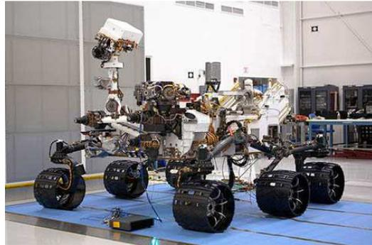
FIGURE 1.4 – Le robot *Curiosity* (JPL/NASA)
