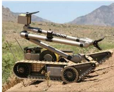
FIGURE 1.10 – Le robot *Packbot* (IRobot)
