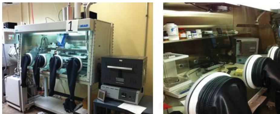
Figure 2.7 Dried-air purged glove box with humidity<1%
