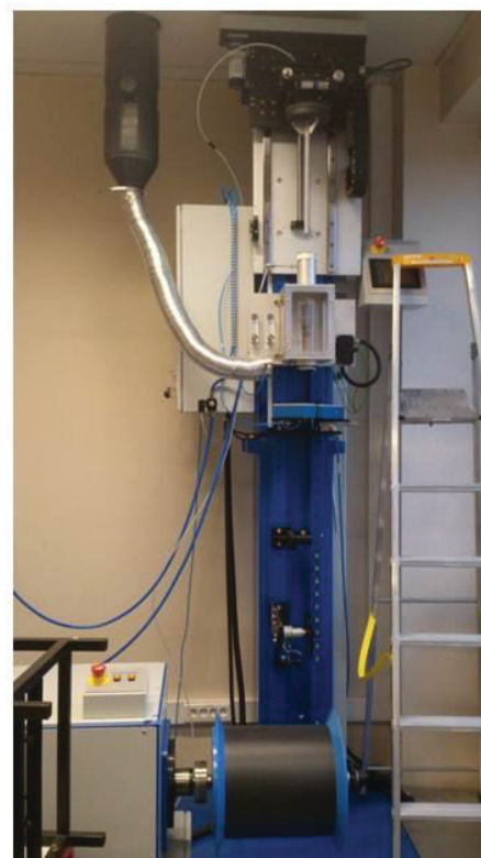
Figure 2.13 Drawing tower facilities at Institut Carnot de Bourgogne, University of Dijon, France – Prof. Frédéric SMEKTALA
