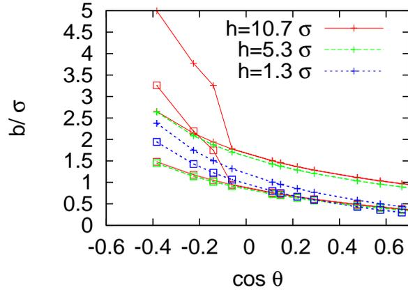
FIGURE 4.4. Slip length  $b$  as a function of  $\cos \theta$  on crenelated rough surfaces for three values of the crenel depth  $h$  (colors). + symbols correspond to parallel slip and  $\square$  symbols to perpendicular slip. Bifurcations ( $h = 10.7\sigma$ ) indicate coexisting CB and W states ( $T = 0.7T_c$ ). Branches with larger  $b$  are CB states.
