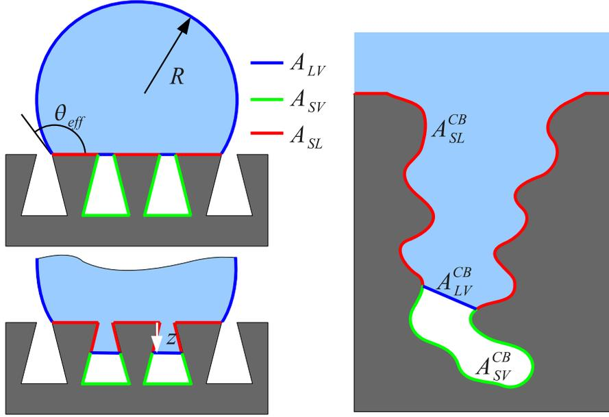
FIGURE 3.5. Left: Schematic sketch of the geometry in the heterogeneous wetting regime. Note that in the Cassie-Baxter theory the drop is assumed to be much larger than the length-scales of the roughness. Right: Heterogeneous wetting situation in an arbitrary rough substrate.  $A_{SL}^{CB} + A_{SV}^{CB} = A_0$
