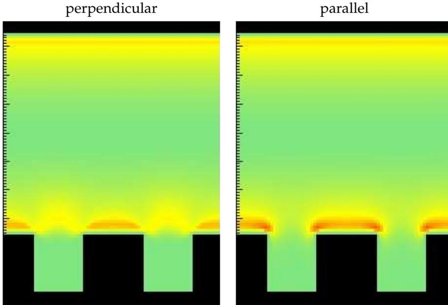
FIGURE 4.7. Dissipation power density for PF in W wetting state: left: perpendicular flow right: parallel flow
