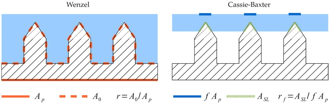
FIGURE 3.1. Corrugated substrate geometry:  $A_0$  is the total substrate surface area,  $A_p$  its projection,  $f$  is the fraction of the projected area, which is wetted, the total roughness factor  $r = A_0/A_p$  and the wetted roughness factor  $r_f$  describes the roughness of the wetted part only.
