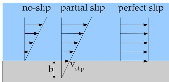
FIGURE 4.1. Navier partial slip boundary condition, the no-slip limit and perfect slip limit
