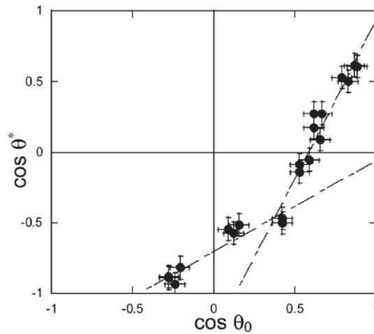
FIGURE 3.8. Wetting diagram of superhydrophobic and omniphobic fractal surface from the Ramos experiment. Figure taken from ref. [250].
