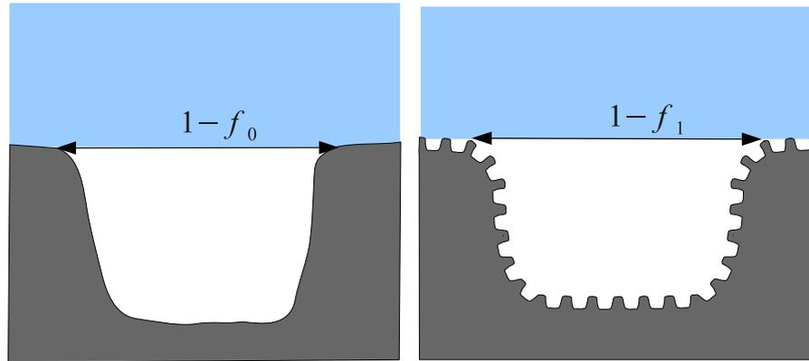
FIGURE 3.6. *Self-affine substrate: Similar corrugation appears at several length-scales, from molecular lengths to capillary length.*
