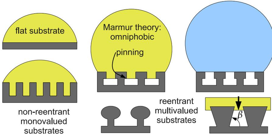
FIGURE 3.3. Examples of mono- and multivalued substrate geometries. Metastability is exploited to gain omniphobicity with multivalued geometries.
