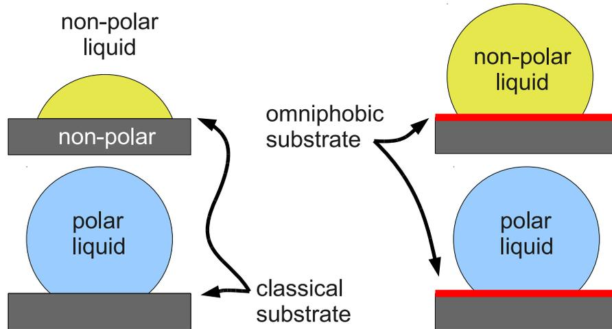
FIGURE 3.2. *Illustration of omniphobicity. A flat and chemically homogeneous surface of e.g. a non-polar substrate material exhibits intrinsic contact angles (CA)  $\theta$  less than  $90^\circ$  for non-polar liquids and CA greater than  $90^\circ$ . An omniphobic substrate is supposed to exhibit repellent behavior for both types of liquids, described by the effective/apparent contact angle.*
