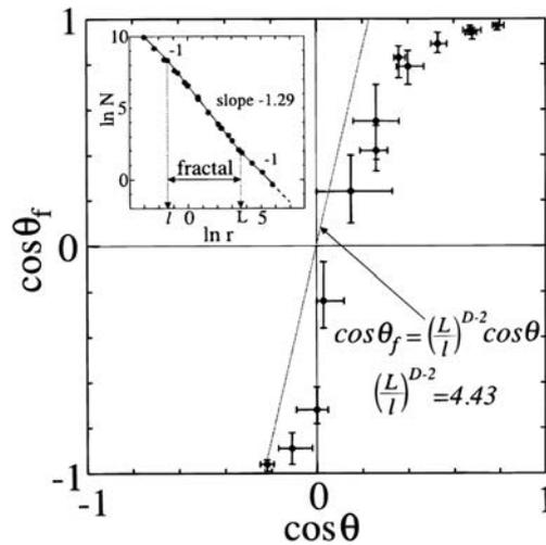
FIGURE 3.9. Wetting diagram of alkylketene dimer fractal surfaces. Figure taken from ref. [235]. Note, the apparent contact angle is denoted  $\theta_f$  here.
