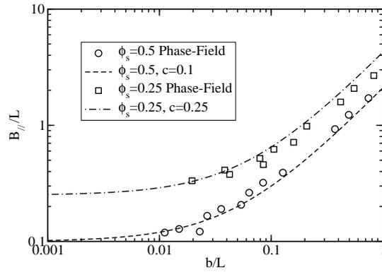
FIGURE 4.8. Scaling law satisfied by  $B_{||}$  as a function of  $b$  and  $L$ . the symbols correspond to the values obtained with the PF model for a crenelated surface, the dashed and dot-dashed lines corresponds to the simple approximation (4.15) for  $\phi_s = 0.25$  and  $\phi_s = 0.5$ . It is remarkable that the obtained values of  $c$  are in quantitative agreement with fig. 12 of ref. [73], though the geometries are different (see text).
