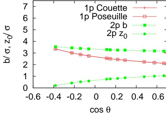
FIGURE 4.2. Slip length  $b$  and wall position  $z_0$  for 1 parameter and two parameter fitting method. Poiseuille and Couette flow give virtually the same result, 2 parameter method (2p) displays wall positions different from 0 and according to this larger slip lengths. Notice for the 2 parameter method:  $z_0 - b = -b_1/a_1$ .
