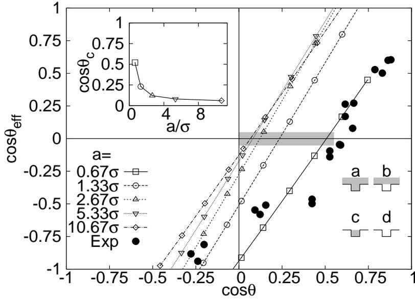
FIGURE 3.12. Wetting diagram:  $W$  branches of monodisperse pillars with pillar width  $a = (0.67, 1.33, 2.67, 5.33, 10.67)\sigma$ ; ( $L - a = h = 13.3\sigma$ ). The insert shows the intrinsic  $\cos\theta$ , where the substrate changes from non-wetting to wetting ( $\cos\theta_c^W$ ) as a function of the pillar width  $a$ . For pillars with only atomic thickness the Wenzel wetting inversion angle  $\theta_c^W$  is comparable to the experimental findings of ref. [250] (solid dots).
