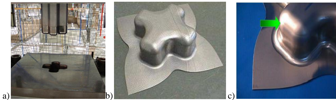
Figure VIII.35: a) The tools used for the cross-die test, b) The final configuration of the deformed specimen, c) necking in the product [ATE 2004].
