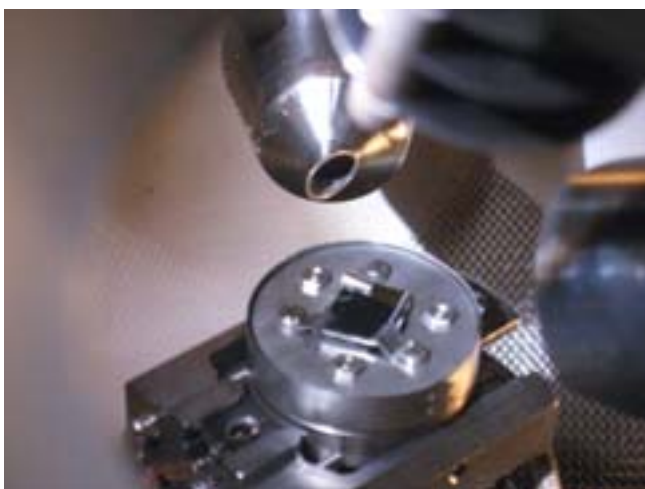
Figure 2.10 Sample holder for the XPS system for low gas pressure/UHV studies
