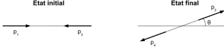
Figure 3.6: Elastic scattering principle characterized by the angle \theta .
