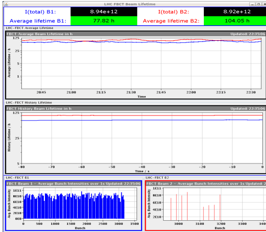
Figure 6.21: Intensities configuration as captured from the LHC op vistar during the 90 m \beta^* ALFA data taking.
