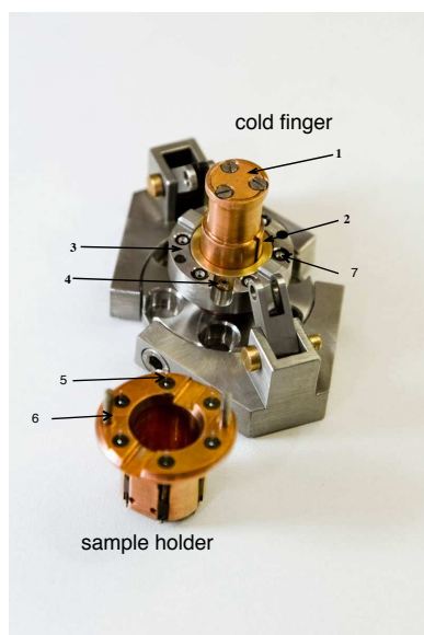
Figure 8.4: New set-up for sample holder with electrical contacts. (1) Temperature sensor cap (2) cold finger (3) Rotating Ring (4) Non-Rotating ring, (5) male electrical pins, (6) transfer pins, (7) female electrical pins. with two 0.9 mm screws fixed on the cold finger.
