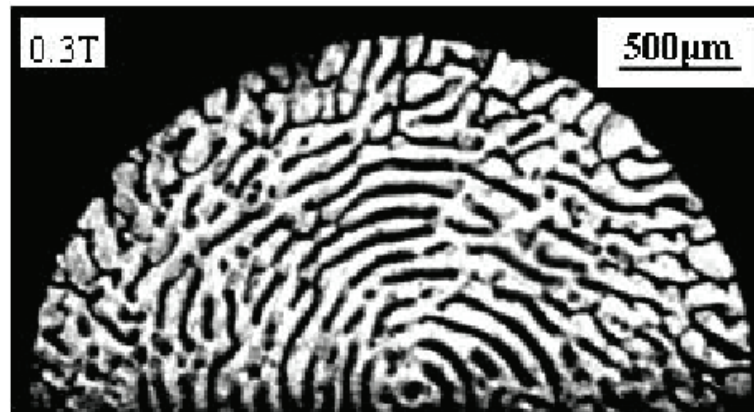
Fig 1-2 Solidified microstructure of Al-0.85wt.%Cu alloy in the mush zone [LI09b]
