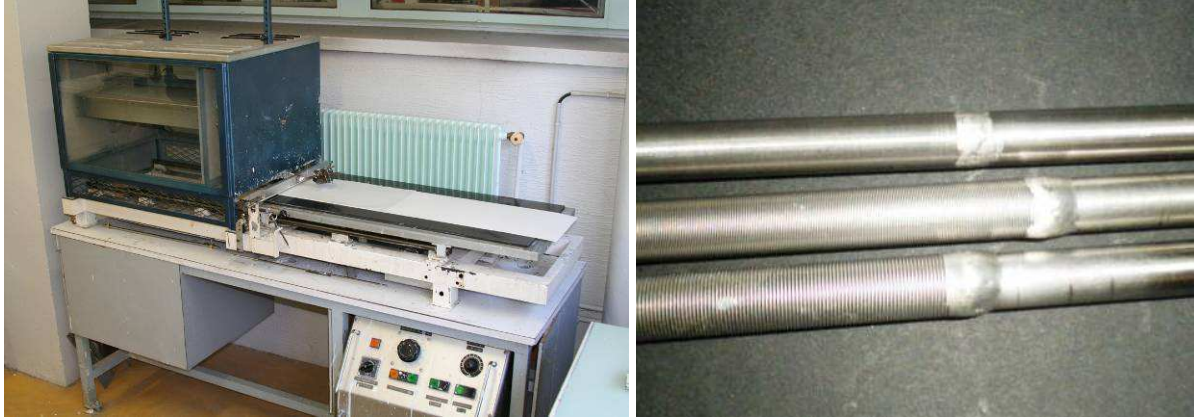
Figure II-13: Laboratory rod coater (left) and several wire wound rods (right).
