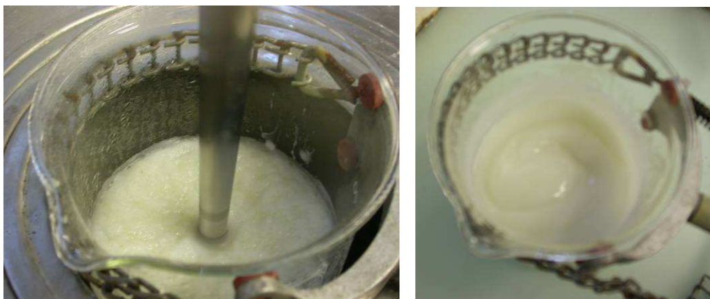
Figure II-12: Solubilisation of PVOH in MFC suspension.
