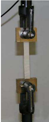
Figure II-22: Tensile test with an Instron device.
