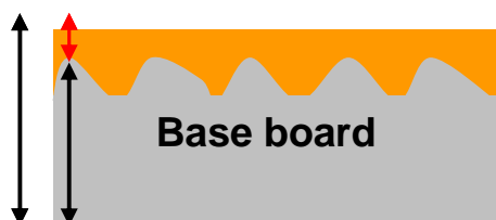
Figure V-16: Effect of the roughness of the uncoated board on the final thickness.
