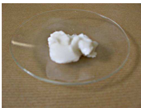
Figure V-6: Photos of MFC suspension at 6.3% after centrifugations.
