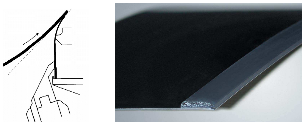
Figure V-28: Principle of the Bent blade [25] (left), photo of DUBLADE Soft-Tip [175].
