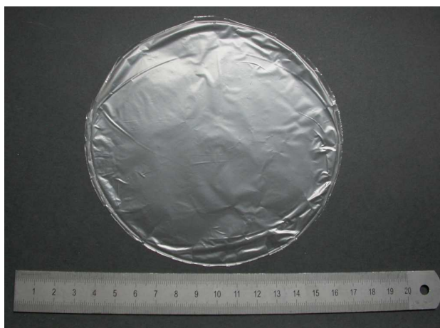
Figure III-46: Visual aspect of TEMPO MFC film. Compared with enzymatic?
