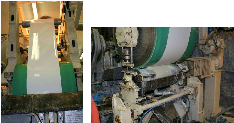
Figure II-16: Wet paper after coating and applicator roll.
