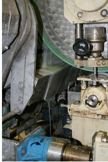
Figure V-26: Overflowing of coating colour.
