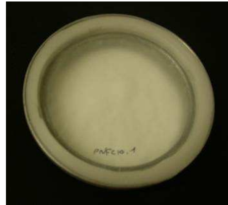
Figure II-24: Dish method to determine the WVTR of samples.
