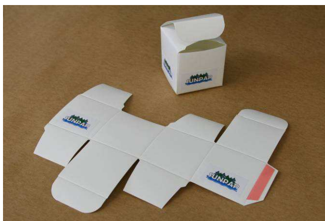
Figure V-61: Production of boxes from coated board samples.
