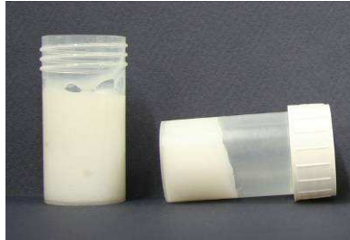
Figure IV-1: Photos of MFC-E-MG suspension at 2 wt%.
