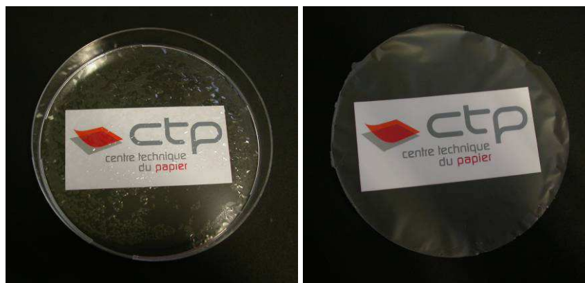
Figure III-54: Films of 30g/m 2 of starch/sorbitol (80/20) (left) and starch/S/MFC (56/14/30) (right).
