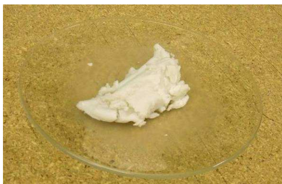
Figure V-9: Visual aspect of MFC concentrated at 10.5 wt% by inverted dialysis.
