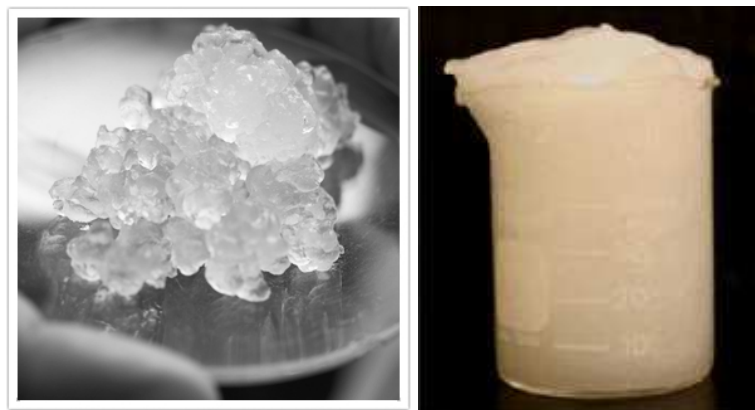
Figure I-28: Photos of carboxymethylated MFC gel [84] (left) and of TEMPO oxidized MFC gel [38] (right).
