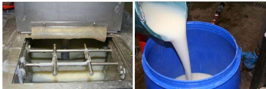
Figure II-14: Preparation of coating colour at pilot scale.
