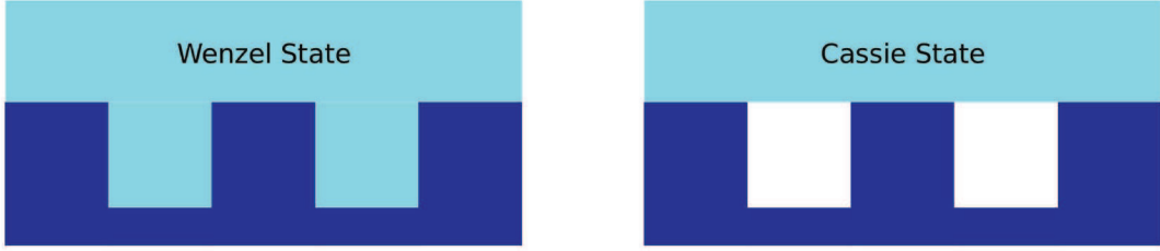
Figure 4.2: Schematic representation of the Wenzel state: water filling the roughness cavities, and the Cassie state: air bubbles trapped inside the cavities.
