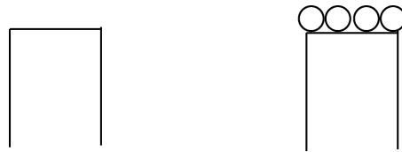
Figure 30: the smooth and “rough” pins made of stainless steel. These pins have the same surface area (in contact with the sock) than the Lorica® pin.
