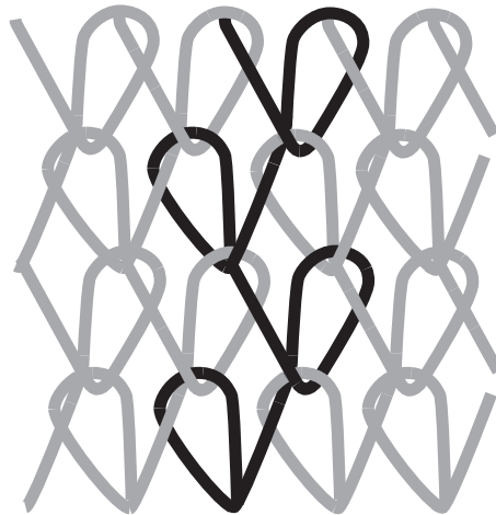
Figure 11: example of warp knitted fabric; 1 and 1 lapping structure.
