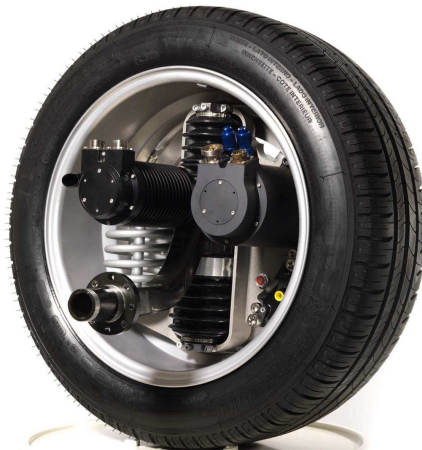
Figure 1.9: An example of in-wheel electric motor system [67].
