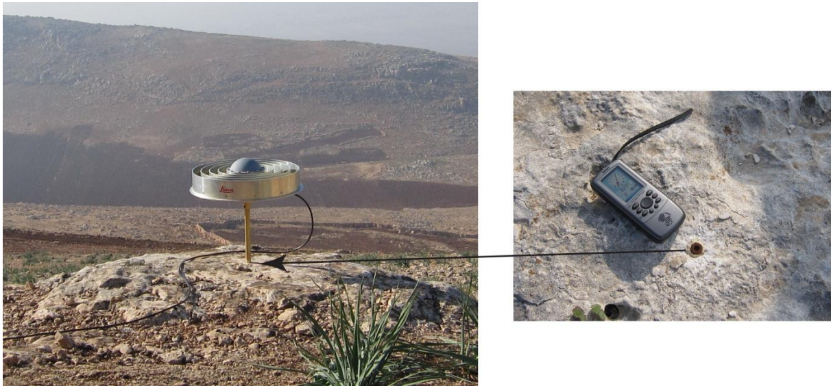
Figure III.6 : Example of GPS monument used in Syria Thales DSNP 6502MK receivers and Leica AT504 Choke Ring Antenna
