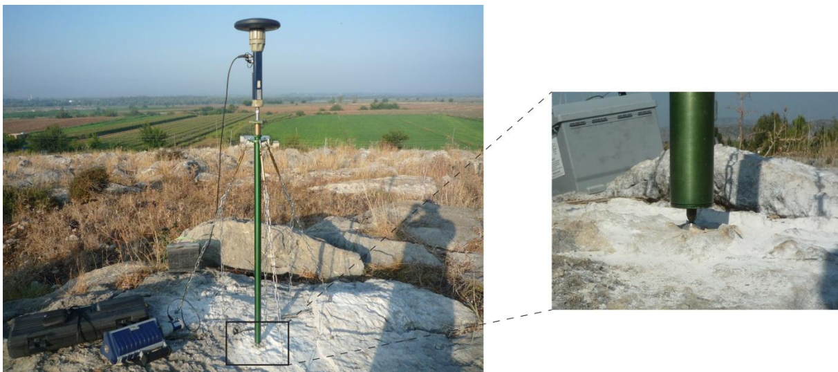
Figure III.5: Example of GPS monument used in Turkey with Thales Z Max receivers and Thales Z Max Ashtech antenna
