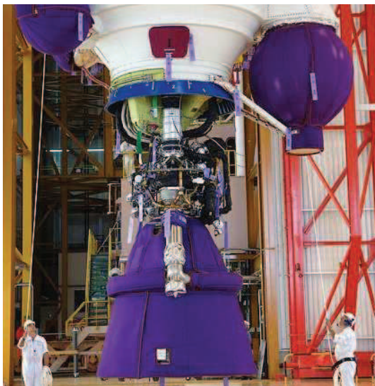
(a) Ariane 5 Vulcain2 engine mounted on the support frame, gimbal and hydraulic actuators
