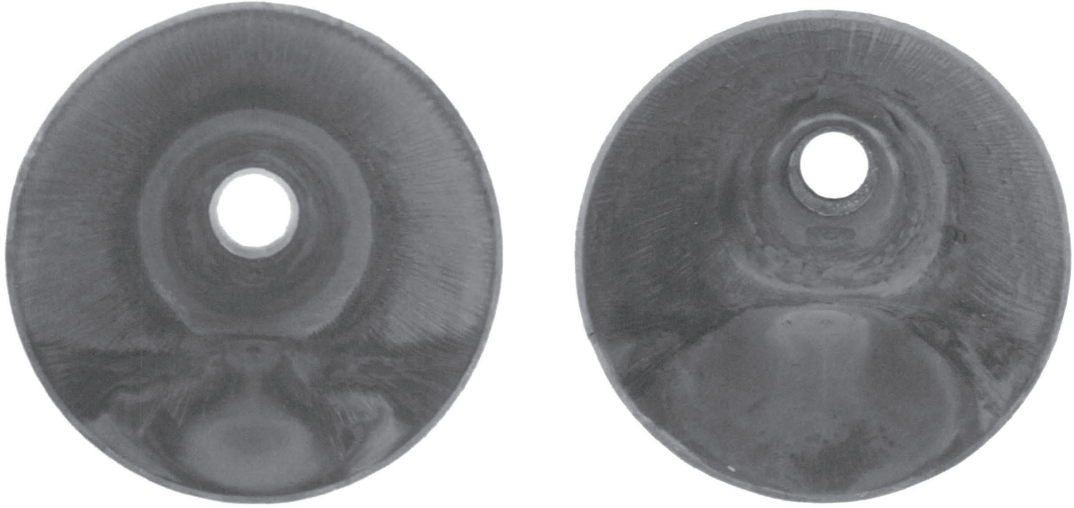
(a) f_m = 0.03 small separation zone and (b) f_m = 0.07 larger separation, no reattachment downstream flow reattachment
