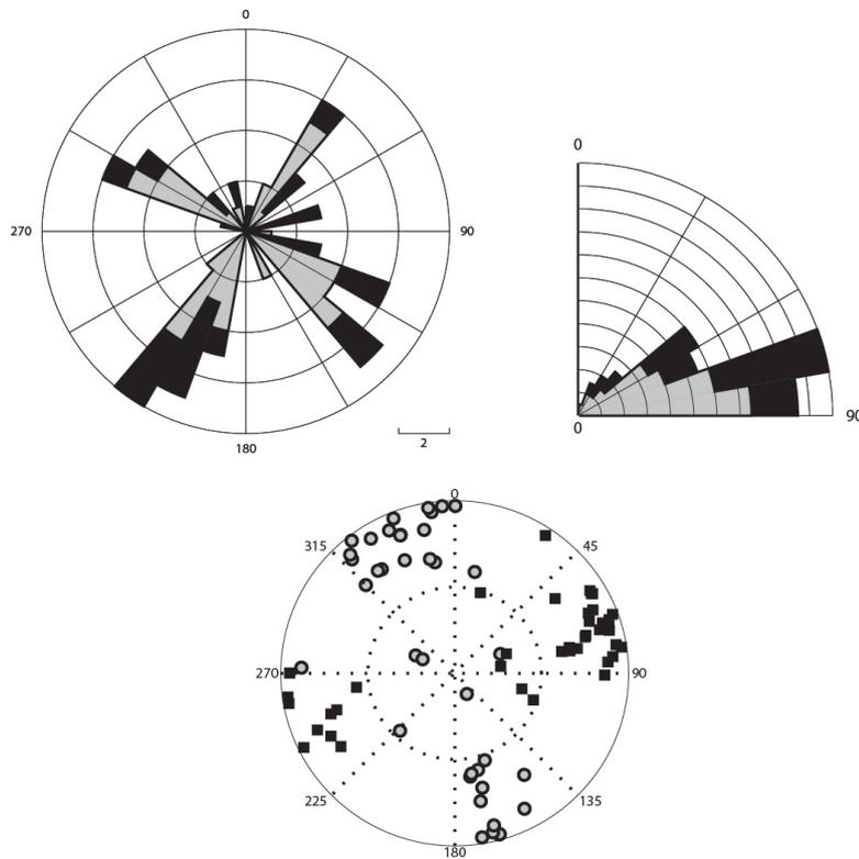
**FIGURE 2.2.4:** *The first line shows the azimuth and dip of the two nodal planes of every focal mechanism (in black). The reduced dataset orientations are shown in grey. At the bottom, the P and T axes of the 39 focal mechanisms are plotted.*
