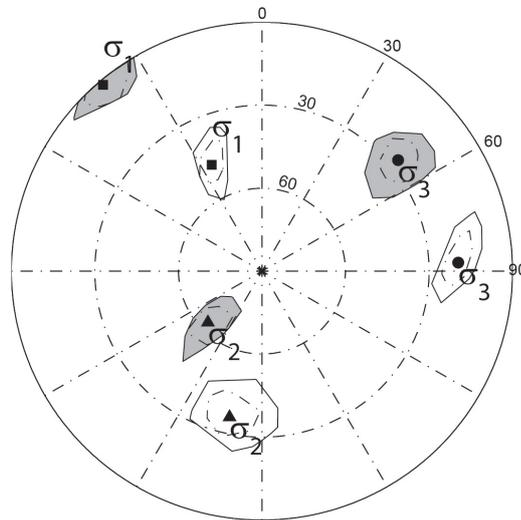
**FIGURE 2.2.11:** *Principal stress directions determined with Julien and Cornet's method using the reduced dataset. Two minimum are found. The solution A yields the principal stress directions with the confidence regions unfilled and the solution B yields the principal stress directions with the confidence regions in grey. See figure 2.2.7 for a description of the figure.*
