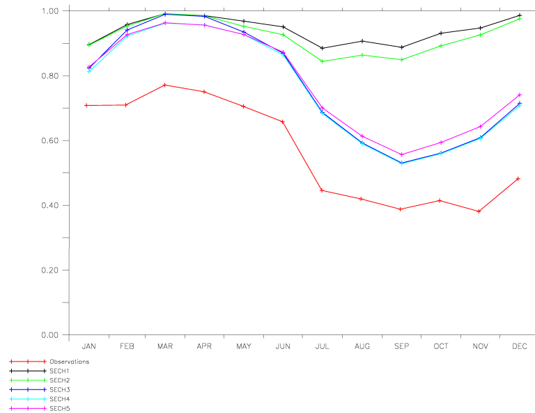
Figure 4.7: MONTHLY MEAN SWI AVERAGED OVER THE EIGHT SELECTED STATIONS, FOR THE MEAN TIME PERIOD 1997-1999, FROM OBSERVATIONS (RED) AND DIFFERENT SIMULATIONS PERFORMED (COLORS).
