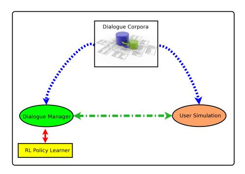
Figure 9.1: Dialogue optimization using RL and user simulation
