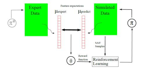
Figure 7.1: User simulation using imitation learning
