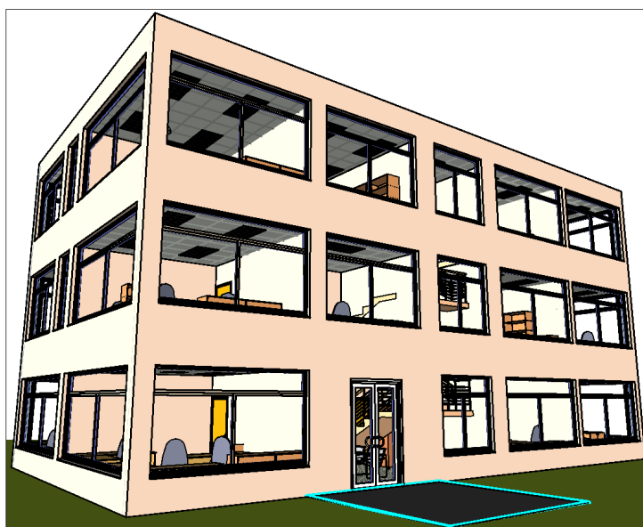
Figure 3.7 Test building representation. This building represents a typical small office building. It consists of 20 zones, its area is approximately 540 m 2 .
