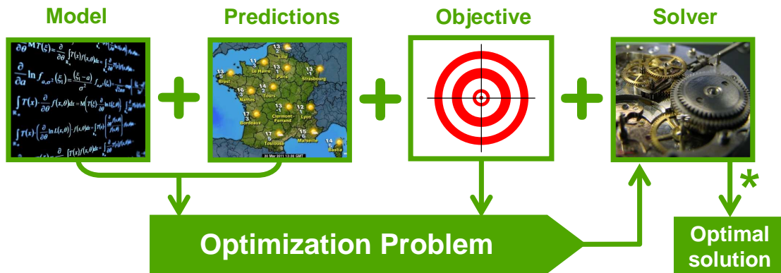
Figure 2.2 Model Predictive Control ingredients in buildings. In building, MPC lies on using a model of the building as well as prediction on disturbances to formulate and solve at each decision instant an optimization problem to find the best sequence of actions which minimizes the cost function (energy, invoice, etc.) and ensure occupant comfort.
