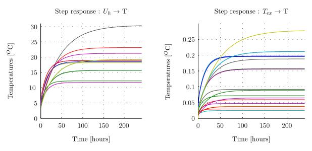
**Figure 3.8** Step response of the 20-zone building. Note that temperature responses exhibit two phases: a fast increase due to air dynamic (clearer on figure 3.9) and a very slow dynamic due to walls dynamic. This generally leads to very ill conditioned problems during identification (see [Malisani et al. 2010]).
