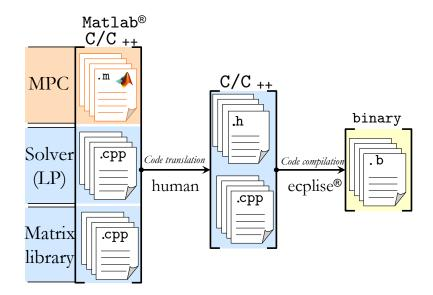
**Figure 4.29** RoomBox implementation steps. The code developed on Matlab has been translated to  $C^{++}$ , then compiled in Eclipse environment.
