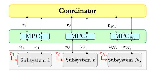
**Figure 6.1** Hierarchical Distributed Model Predictive Control: the coordinator manages the subsystems allowable resource profiles  $\{\mathbf{r}_{\ell,k}\}_{\ell \in S}$  to ensure that the global constraint (6.2.5) is always verified.
