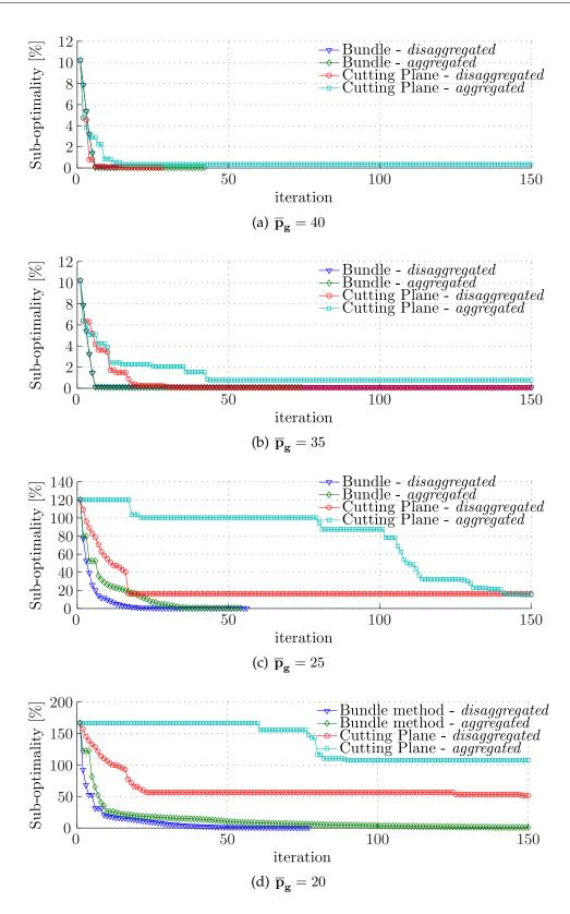
**Figure 7.7** Illustration of the bundle algorithm effectiveness for increasingly constrained optimization problems.
