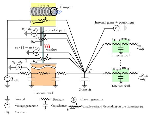
**Figure 3.4** Thermal-electrical analogy - simplified circuit. The bilinearity of the model is due the varying resistors involved in the model (ventilation  $u_v$  and blind position  $u_b$ ) as well as the products involved in the window heat transfer model ( $u_b \cdot \phi_g$ ).
