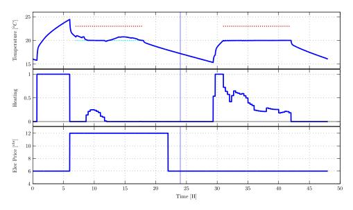
**Figure 2.4** Illustration of the usage of MPC with variable price energy. Note that during the first day the building is overheated during the off-peak period (before 6 a.m.), the second day the energy price is constant and therefore no overheating is performed (an optimal start is implemented).
