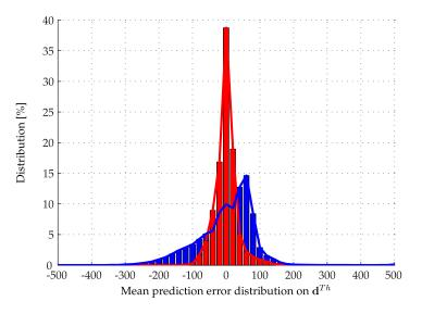
**Figure 4.6** Prediction errors comparison between the proposed prediction mechanism (red). In blue: employing the current observed value over the whole prediction horizon( $d^+ = d$ ). One can note that prediction is improved.
