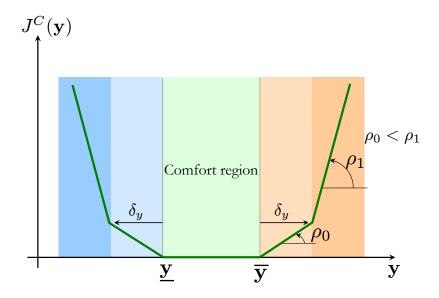
**Figure 4.3** Discomfort function used in the optimization problem 4.1: The discomfort function is parametrized by  $\rho_0$ ,  $\rho_1$  and  $\delta_y$  which represents a reasonable bound violation.
