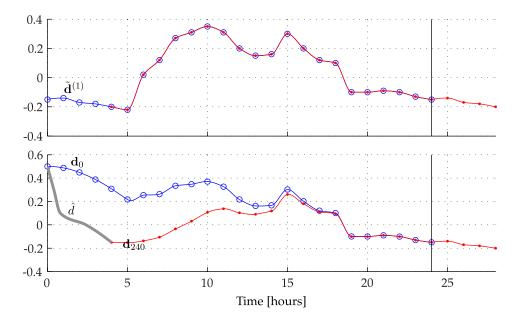
**Figure 4.5** Disturbance prediction principle. The predicted disturbance is based on the current estimation of the disturbance provided by the state observer (*d*) (see the extended system (4.5.4)) as well as past observed disturbances during previous days  $\tilde{\mathbf{d}}^{(1)}$ .
