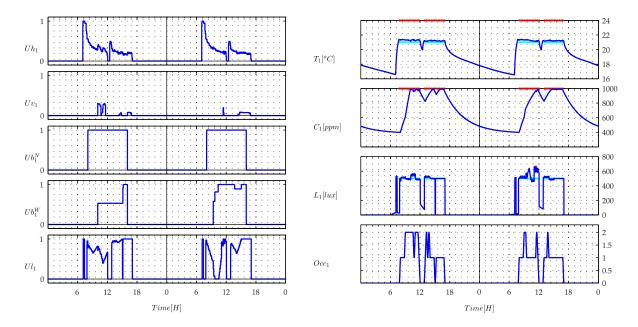
**Figure 4.11** Zone model predictive controller validation - illustrative behavior in an office. Note that temperature bounds, CO<sub>2</sub> and lighting bounds are respected.
