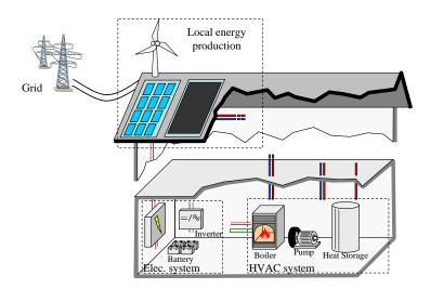
Figure 2.6 Illustration of the main equipment controlled at the energy layer.
