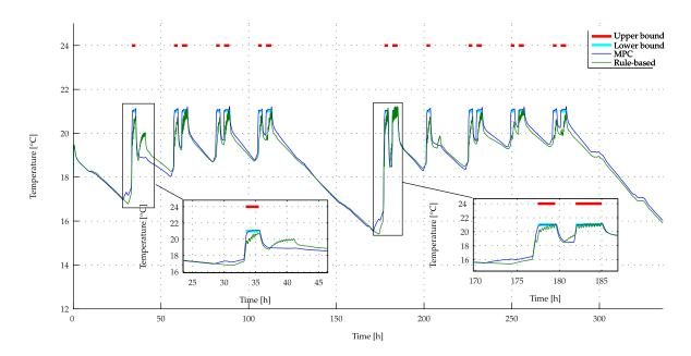
**Figure 4.24** MPC vs. Rule-based control - temperature profile in a meeting room during the two first weeks. Observe that control performances with MPC are much better.
