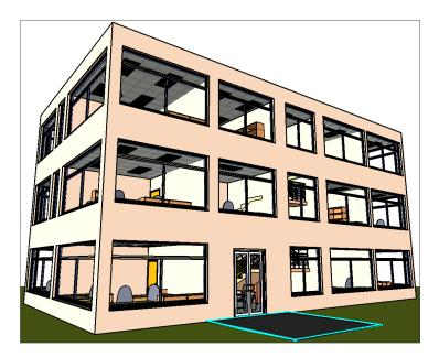
**Figure 3.7** Test building representation. This building represents a typical small office building. It consists of 20 zones, its area is approximately 540 m<sup>2</sup>.
