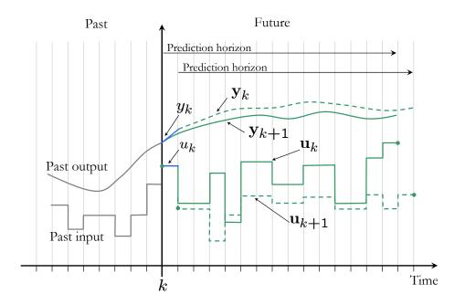
**Figure 2.1** Receding horizon principle: at each decision instant a new optimal control trajectory  $u_k$  is computed, only the first element of the sequence  $(u_k)$  is implemented, and so on.
