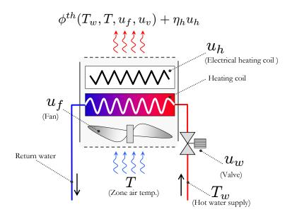
**Figure 5.2** Fan Coil Unit representation. There are two heating coils: an electrical heating coil and a heat exchanger. The fan speed and the valve opening define the heat exchange coefficient  $\phi^N$  (see eq. (5.2.1)).
