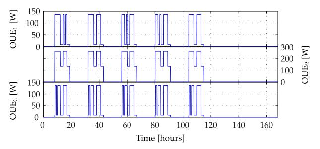
**Figure 3.12** Other Usage of Electricity (OUE) profiles. OUE consist of noncontrollable electric consumption in the zone, their integration in the simulation tool is of particular importance for their heat production.
