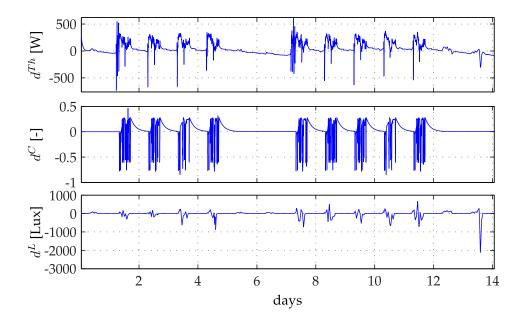
**Figure 4.4** Estimated disturbances on two weeks. Note the periodicity of the disturbances. The flat parts ( $d^{Th}$  and  $d^{C}$ ) correspond to week-ends. The other parts correspond to occupied periods. The daily shape of estimated heat flux is due to occupants and equipment heat production, as well as heat exchanges between zones.
