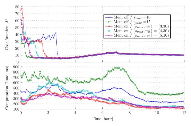
**Figure 7.8** Comparison of performance of the DMPC algorithm with and without distributed-in-time feature during the first 12 [h]: in the presented case study, this enables to reduce the computational time by more than 60 % for quite similar performances in terms of cost function decrease. The mean computational time of the centralized solution is in this case 1.23[s].
