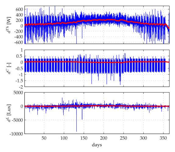
**Figure D.1** Estimated disturbances during one year (blue: estimated, red: filtered). Note that the estimated heat flux  $d^{Th}$  increases during summer due to the fact that adjacent zones temperatures are larger (which results in receiving more heat).
