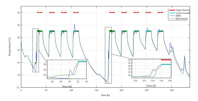
**Figure 4.23** MPC vs. Rule-based control - temperature profiles in an office during the two first weeks. The two rectangles correspond to optimal starts after a long vacancy period.
