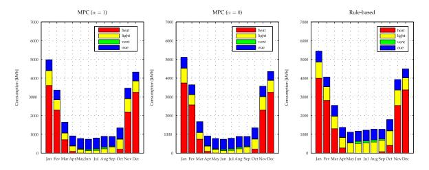
**Figure 4.22** MPC vs. RB monthly energy consumptions. Note that introducing uncertainty in forecast induces more energy consumption but still less than with rule-based control.
