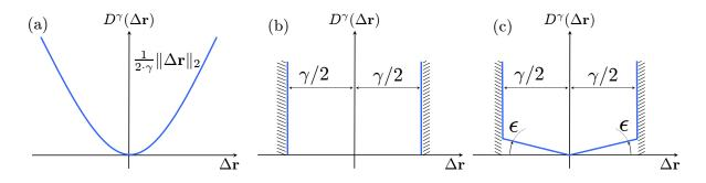
**Figure 6.3** Stabilization terms. (a): quadratic stabilization term. (b): trust region. (c): stabilized trust region.
