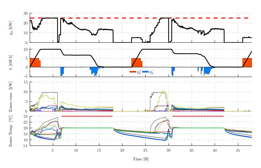
**Figure 7.9** DMPC ( $s_{max} = 3$  iterations with memory) with battery management and power limitation for a 20 zones building. Note that the closed-loop profiles are slightly different from those obtained with a centralized control (figure 7.10). However, invoice and comfort are quasi-similar.
