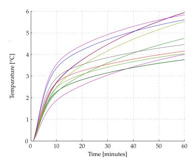
**Figure 3.9** Step responses  $(U_h \rightarrow T)$  during the first hour (figure 3.8). Note that electrical heaters may generate a temperature increase comprised between 4 and 6 [°C] after one hour.
