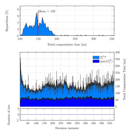
**Figure 7.11** Computation time. Results obtained on an Intel<sup>®</sup> Core<sup>(TM)</sup> *i*7 CPU X920 @ 2.00 GHz, 3.23 Go RAM. ILOG CPLEX 12.1 solver was used.
