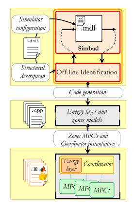
**Figure 4.21** MPC integration in SIMBAD - workflow. The off-line identification procedure is described in chapter 3. Coordinator and energy layer will be discussed in chapter 7.
