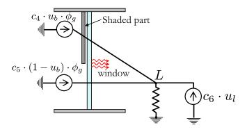
Figure 3.6 Simplified indoor illuminance model - electrical analogy
