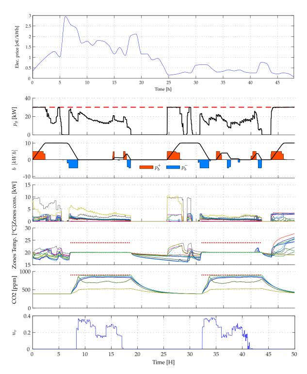
**Figure 7.13** DMPC with a shared input actuator. Notice that the CO<sub>2</sub> level is decreased in some zones to meet the requirements on other zones (since a unique actuator affects the whole zones). Notice also that the battery is basically used to store energy during low price periods in order to redistribute it to the zones when energy price is higher.
