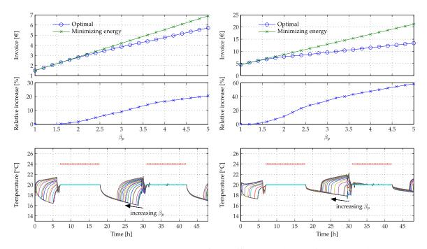
**Figure 4.14** Invoice minimization for different values of  $\beta_p$  with the same zones but with a different heater dimensioning (heaters powers is reduced by 50 %). The first sub-plot corresponds to the invoices obtained for different values of  $\beta_p$  (optimal) and the corresponding invoice if minimizing energy. The last sub-plot corresponds to the optimal temperature trajectories.
