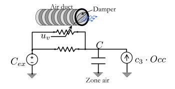
**Figure 3.5** Simplified CO<sub>2</sub> model - electrical analogy. The model is bilinear due to the existence of input-output product  $u_v \cdot (C - C_{ex})$ .
