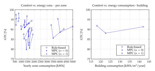
**Figure 4.26** MPC vs. Rule-based control. Notice that bad weather forecast  $(\alpha = 0)$  mainly induces less comfort in the zones and generally more energy consumption.
