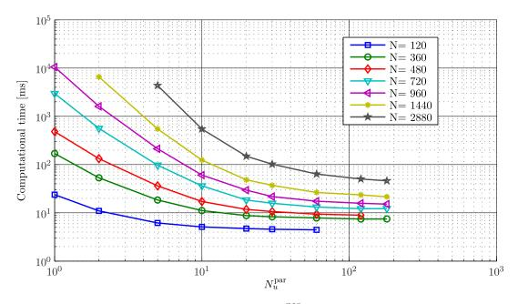
**Figure 4.9** Computational time vs.  $N_u^{\text{par}}$  for increasing horizon lengths  $(N_u^{\text{par}} = N_y^{\text{par}})$ . Note that the computational burden obviously decreases with increasing  $N_u^{\text{par}}$ . However this leads to a loss in performance (see table 4.1, page 71), illustrating the trade-off between performance and computational burden.
