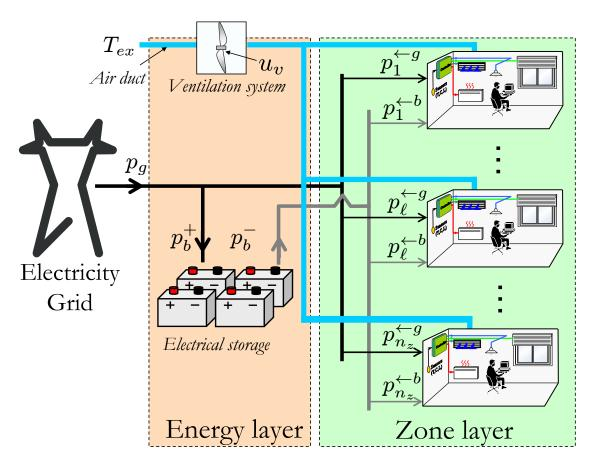
**Figure 7.12** Handling shared actuators between zones with DMPC. The ventilation system impacts all the zones simultaneously, therefore its management should take into account all the zones *needs* in terms of fresh air. The simulation results are reported in figure 7.13
