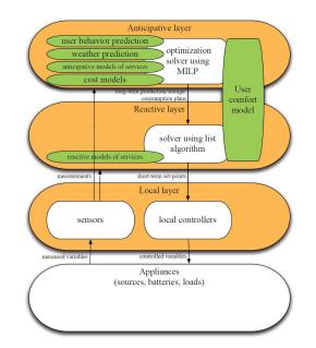
**Figure 2.8** MAHAS system: the system has 3 layers, the highest layers correspond to slower dynamics [Ha et al. 2008]
