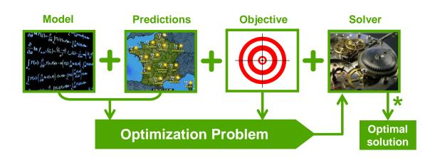
**Figure 2.2** Model Predictive Control ingredients in buildings. In building, MPC lies on using a model of the building as well as prediction on disturbances to formulate and solve at each decision instant an optimization problem to find the best sequence of actions which minimizes the cost function (energy, invoice, etc.) and ensure occupant comfort.
