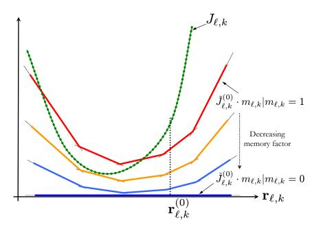
**Figure 6.4** Effect of the memory factor on the first approximation of the function. For decreasing memory factors the initial approximation  $J_{\ell,k}^{(0)}$  keeps less information but on the other hand prevents the optimal solution from being excluded from the search domain.
