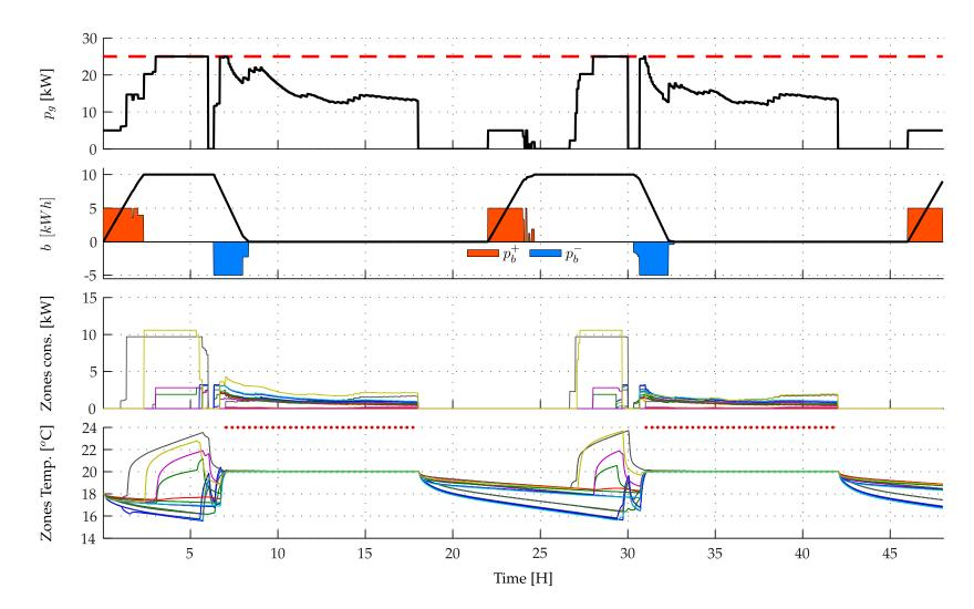
**Figure 7.10** Centralized control with battery management and power limitation on a 20-zone building. These results have to be compared with those obtained using the DMPC algorithm (figure 7.9)
