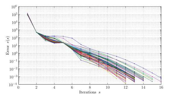
**Figure 4.7** Fixed-point algorithm convergence. Evolution of the error e(s) for 100 randomly generated initial guesses  $\mathbf{u}_k^{(0)}$ . The threshold parameter  $\eta = 10^{-4}$ . One can see that even when starting from quite unrealistic profiles, the algorithm always converges. Moreover, the error decreases monotonically.
