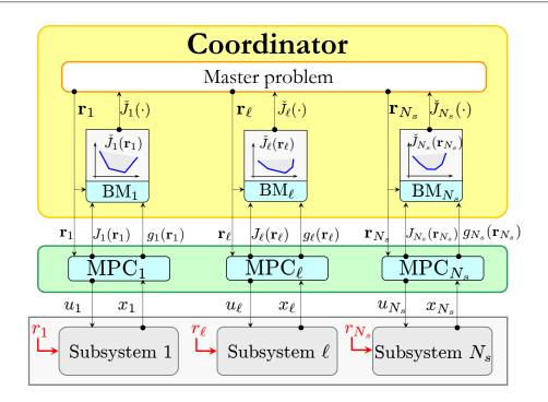
Figure 6.5 Hierarchical Distributed Model Predictive Control scheme.
