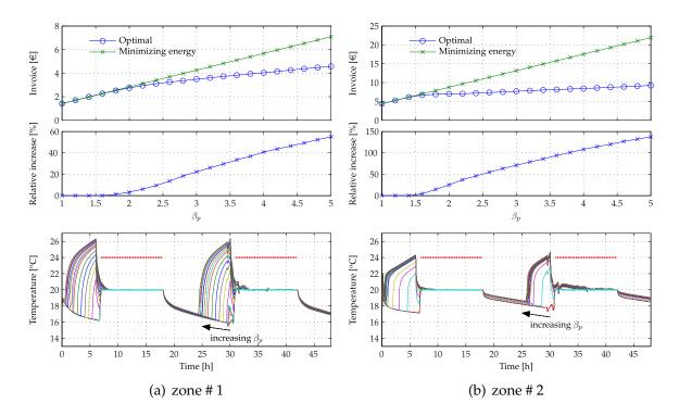
**Figure 4.13** Invoice minimization for different values of  $\beta_p$ . The first subplot corresponds to the invoices obtained for different values of  $\beta_p$  (optimal) and the corresponding invoice if minimizing energy. The last sub-plot corresponds to the optimal temperature trajectories.
