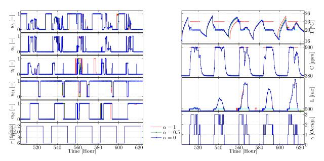
**Figure 4.20** Simulation results with uncertainties on weather ( $\alpha = \{0, 0.5, 1\}$ ) and occupation profile. Notice that comfort bounds on the three controlled variables are always respected.
