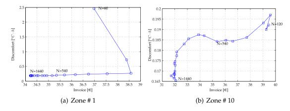
**Figure 4.15** Impact of horizon length on performances for two zones in a building. Notice that sensitivity of the zones regarding horizon length is sensibly different. For the first zone small horizon lengths lead to discomfort while for the second, this only reduces energy usage.
