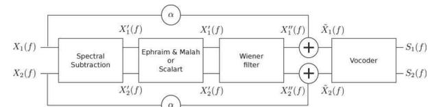
Figure 1. Block diagram of the signal processing
