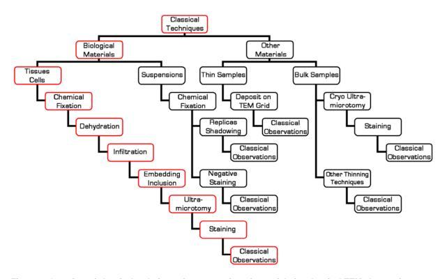
Figure 9: Overview of classical techniques for preparation of materials for classical TEM observations.
