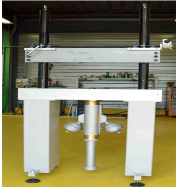
FIGURE 1.1: High performance hydraulic test bench
