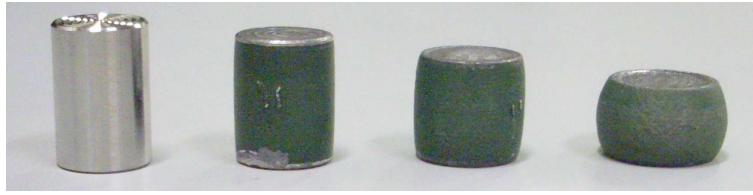
Figure 4.24: Partial compression at strain \epsilon = 0.11 , \epsilon = 0.36 and \epsilon = 0.69
