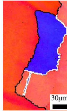
(b) Copper bicrystal deformed at T = 923K , \dot{\epsilon} = 4.2.10^{-4}s^{-1} , \epsilon = 0.15 [112]
