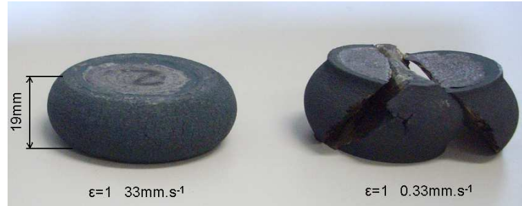
Figure 3.14: Compression of 33mm diameter L-605 samples at T < 1280^{\circ}\text{C} : on the left compression at speed 33\text{mm.s}^{-1} \epsilon = 1 , on the right compression at speed 0.33\text{mm.s}^{-1} until rupture
