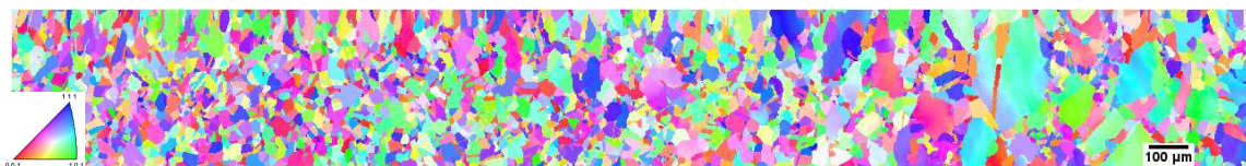
(a) IPF map along the longitudinal axis: left=middle of the sample, right=edge of the sample
