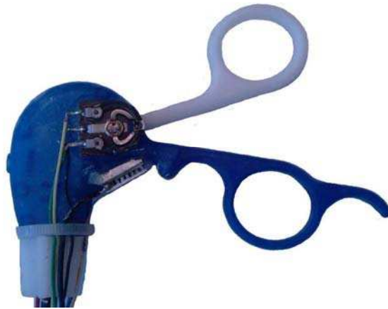
Figure 5.8: Handle sensorization for grasping angle sensing.
