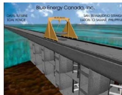
Figure 1.43. La structure "tidal bridge" ©[BEN-09]
