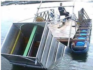
Figure 1.37. Prototype Darrieus caréné ©[TEN-09]
