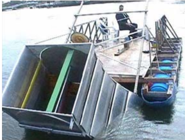
Figure 1.37. Prototype Darrieus caréné ©[TEN-09]
