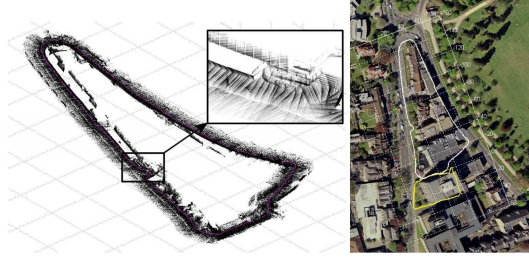
(b) An example metric map built by a robot. (courtesy of Paul Newman, D. Cole, and K. Ho)
