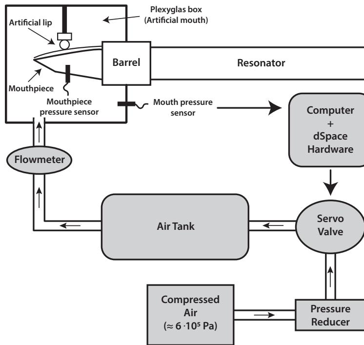
Figure 5.3 – Principle of the pressure controlled artificial mouth.
