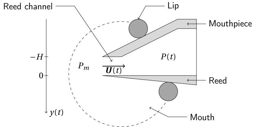
**Figure 4.2 –** Schematic diagram of a single-reed mouthpiece used in Schumacher's model.  $U$  is the flow created by the pressure imbalance  $\Delta P = P_m - P$  between the mouth and the bore,  $y$  represents the displacement of the tip of the reed relative to its equilibrium position and  $H$  is the displacement when the reed is closed.
