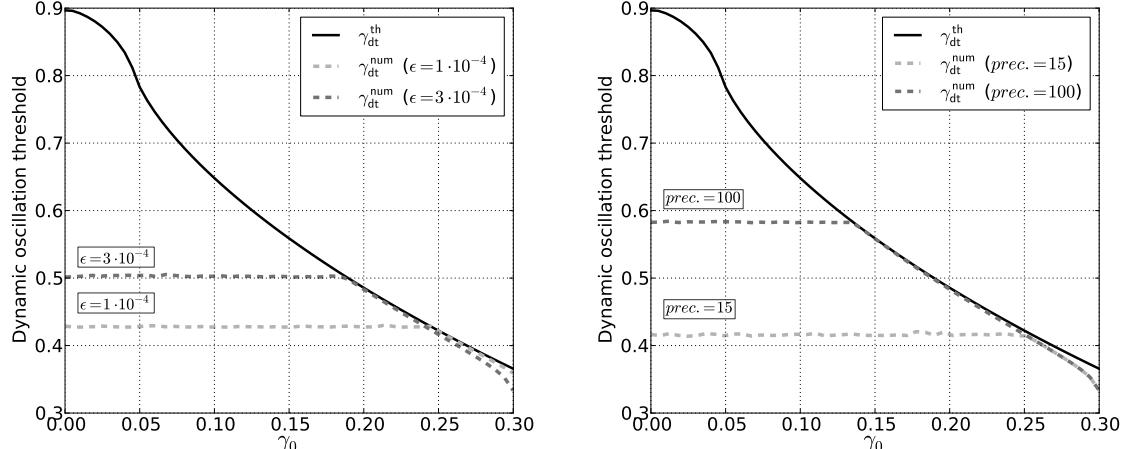
**Figure 3.2** – Plot of  $\gamma_{dt}$  as a function of the initial condition  $\gamma_0$ . Solid lines are the theoretical prediction  $\gamma_{dt}^{th}$  calculated from equation (3.10). Dashed line represent the values  $\gamma_{dt}^{num}$ .
