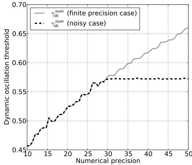
**Figure 3.3** – Comparison of the dynamic threshold  $\gamma_{dt}^{num}$  obtained in numerical simulations of a clarinet model in finite precision case (3.8) and noisy case (3.11) with a noise of level  $\sigma = 10^{-30}$ . The dynamic threshold of oscillation obtained over an average of 20 runs is plotted against the precision used in the simulations, showing that beyond a precision of about  $\sigma$ , the system affected with noise is insensitive to the precision.
