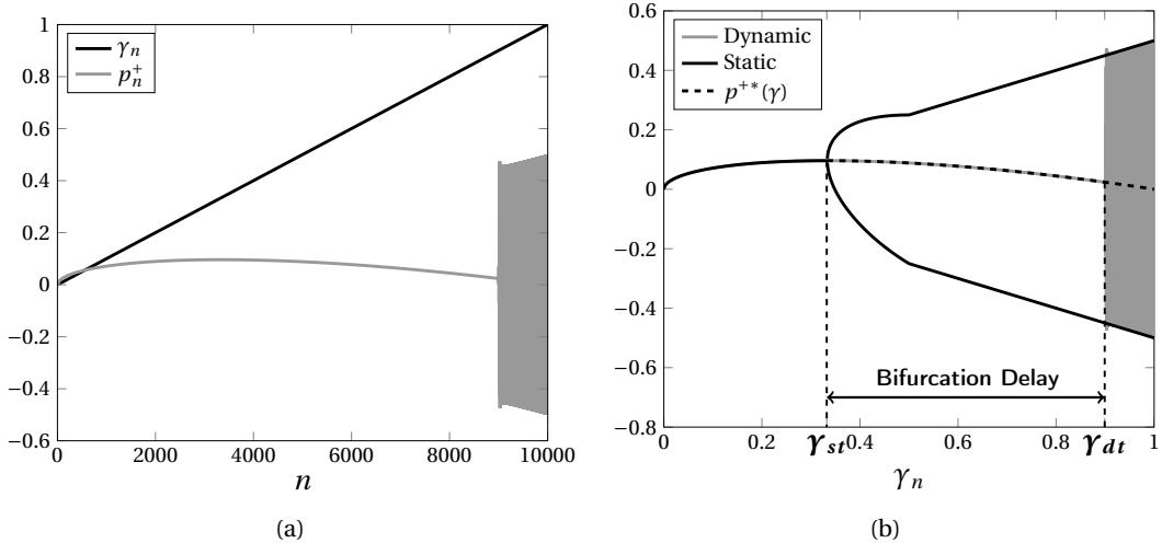
**Figure 2.5 –** (a) Time evolution of the series  $p_n^+$  and of the control parameter  $\gamma_n$ . (b) Comparison between the series  $p_n^+$  and the static bifurcation diagram as a function of  $\gamma_n$ .  $\zeta = 0.5$ ,  $\epsilon = 10^{-4}$ ,  $\gamma_0 = 0$  and  $p_0^+ = G(0, \gamma_0)$ .
