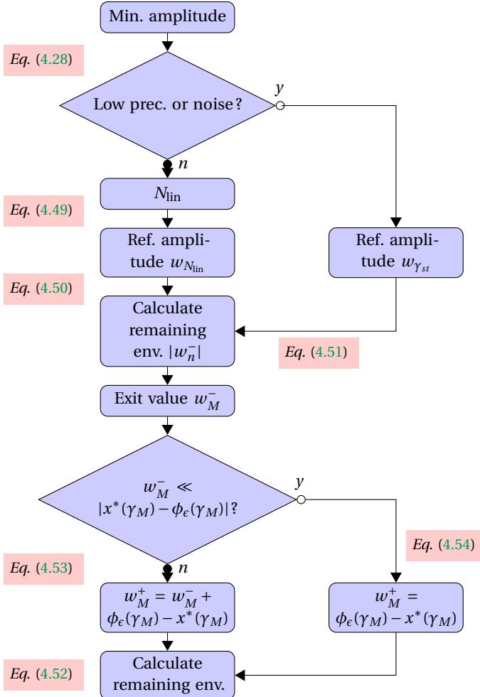
Figure 4.15 – Algorithm for determination of envelope
