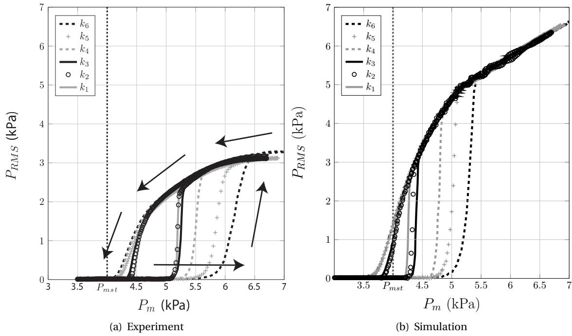
**Figure 5.9** –  $P_{RMS}$  as a function of  $P_m$  for each value of the slope  $k$ . (a) Experimental signals, (b) signals generated by the numerical simulation of the model with parameters  $\zeta$  and  $P_M$  estimated experimentally (cf. section 5.2.4.1) as well as the measured blowing pressure signal  $P_m(t)$ . Arrows represent the direction of the mouth pressure time evolution and highlight an hysteretic cycle.
