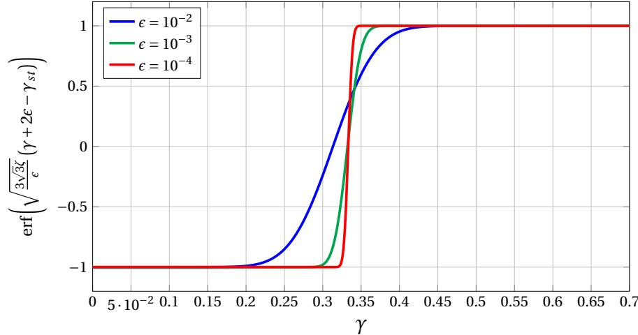
Figure 4.13 – Graphical representation of the function  $\text{erf}\left(\sqrt{\frac{3\sqrt{3}\zeta}{\epsilon}}(\gamma + 2\epsilon - \gamma_{st})\right)$  as a function of  $\gamma$  as for  $\zeta = 0.5$  and for three different values of the slope  $\epsilon$ .
