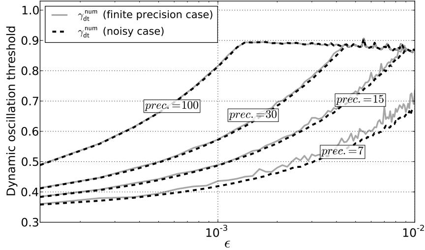
**Figure 3.4** – Comparison between  $\gamma_{dt}^{num}$  computed for *finite precision cases* and for *noisy cases*. For both cases and for each value of  $\epsilon$  we compute the average of the signals  $w_n = p_n^+ - \phi(\gamma_n)$  obtained over 20 runs. Then,  $\gamma_{dt}^{num}$  is calculated on the resulting signal. The numerical precisions used to simulate the finite precision cases are 7, 15, 30 and 100 decimal digits.  $\gamma_0 = 0$ .
