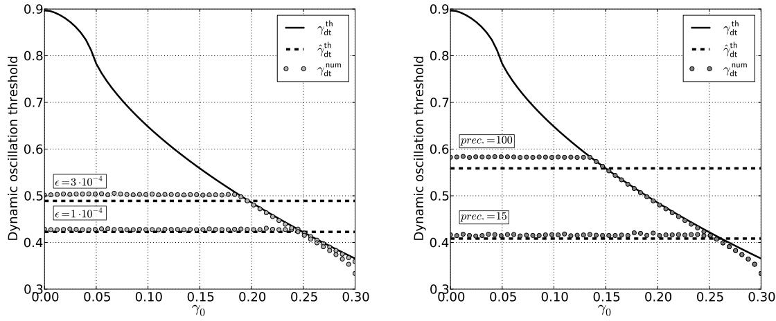
(a) Numerical precision is fixed (prec. = 50).  $\hat{\gamma}_{dt}^{th}$  and (b) The increase rate of  $\gamma$  is fixed ( $\epsilon = 3 \cdot 10^{-4}$ ).  $\hat{\gamma}_{dt}^{th}$  and  $\gamma_{dt}^{num}$  are computed for  $\epsilon = 10^{-4}, 6 \cdot 10^{-4}$ .  $\gamma_{dt}^{num}$  are computed for numerical precisions equal to 15 and 100.
