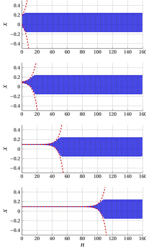
**Figure 4.6** – (—) Time evolution of the outgoing pressure  $x$ , solution of equation (4.9) for different values of its initial value  $x_0 = x^* + w_0$ , from top to bottom :  $w_0 = 0.1$ ,  $w_0 = 0.01$ ,  $w_0 = 10^{-5}$  and  $w_0 = 10^{-10}$ . (---) Exponential envelope deduced from the function (4.17).
