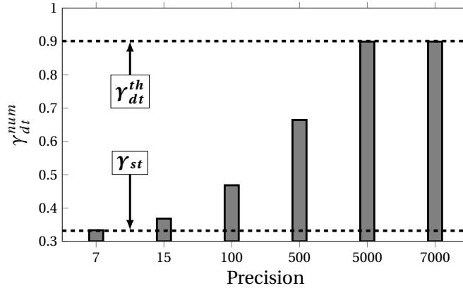
**Figure 2.9** – Graphical representation of  $\gamma_{dt}^{num}$  for different precisions (prec. = 7, 15, 100, 500 and 5000) and for  $\epsilon = 10^{-4}$ . Results are also compared to analytical static and dynamic thresholds :  $\gamma_{st}$  and  $\gamma_{dt}^{th}$ .  $\zeta = 0.5$  and  $\gamma_0 = 0$ .
