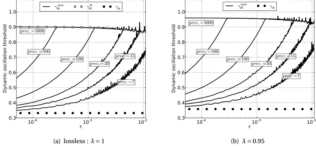
**Figure 3.1** – Graphical representation of  $\gamma_{dt}^{num}$  for different precisions (prec. = 7, 15, 30, 100, 500 and 5000) with respect to the slope  $\epsilon$  and for  $\gamma_0 = 0$ . Results are also compared to analytical *static* and *dynamic* thresholds :  $\gamma_{st}$  and  $\gamma_{dt}^{th}$ . (a) lossless model :  $\lambda = 1$  and (b) typical losses in a cylindrical clarinet,  $\lambda = 0.95$ .
