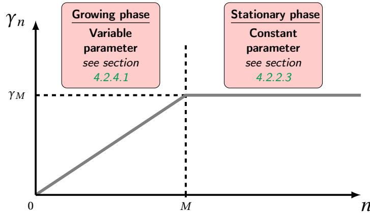
**Figure 4.14** – Schematic representation of the time profile of the control parameter  $\gamma$  : linear growth at a constant rate  $\epsilon$  (the "growing phase") followed by an arbitrary period where it is kept constant at a value  $\gamma_M$ . The instant at which this transition happens is given by the iteration number  $M$  (the "stationary phase").
