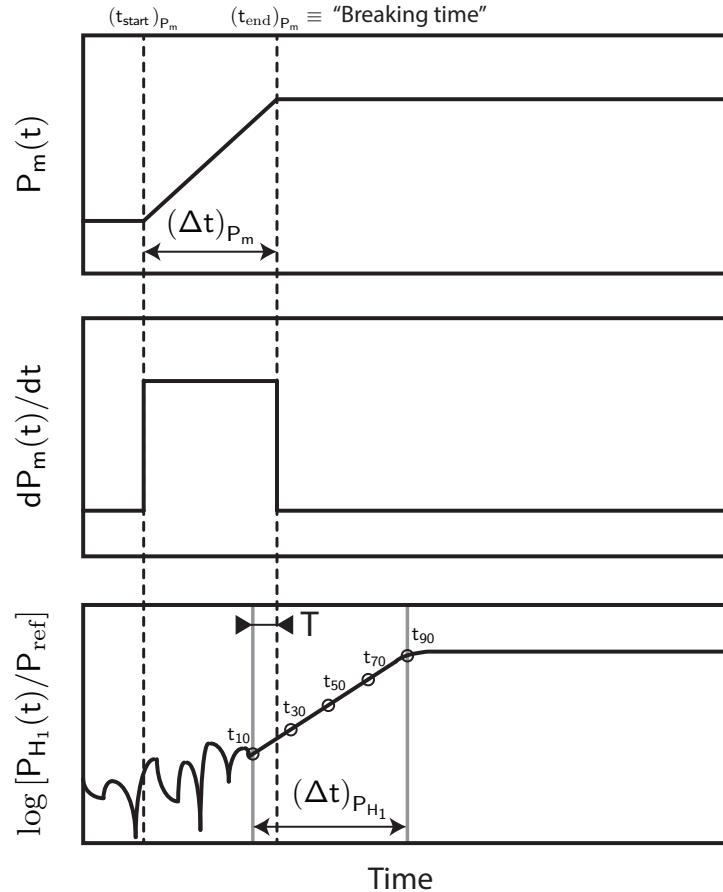
**Figure 5.13 –** Shematic representation of (a) the blowing pressure  $P_m$  and (b) its first time derivative. Dashed lines demarcate the duration  $(\Delta t)_{P_m}$  of the transient of  $P_m$ . (c) Schematic representation of  $\log[P_{H_1}(t)]$ . Gray lines depict the duration  $(\Delta t)_{P_{H_1}}$  of the onset transient of the pressure  $P$  inside the mouthpiece. The duration  $T$ , defined by equation (5.21), is also represented.
