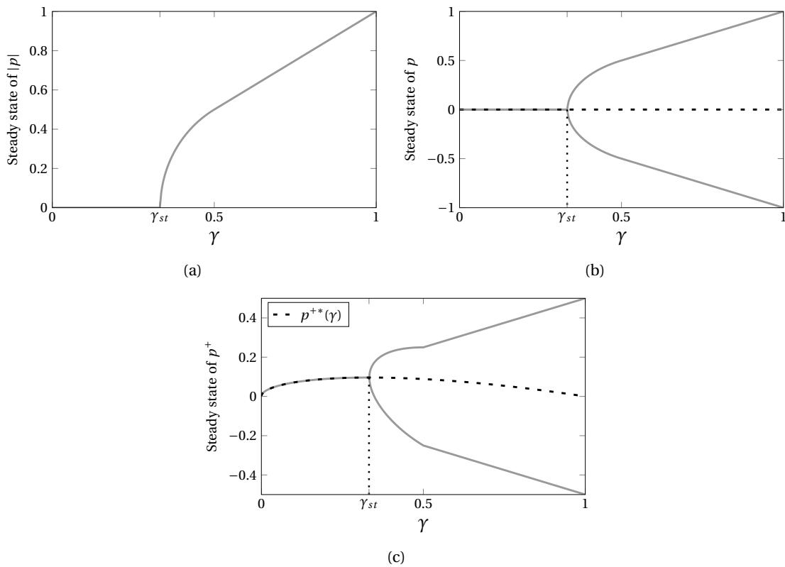
**Figure 2.3** – Graphical representation of the static bifurcation diagrams for  $\zeta = 0.5$ . Diagrams based on variables (a)  $|p|$ , (b)  $p$  and (c)  $p^+$ . The dashed line represents the curve of the static regime, corresponding to the fixed point  $p^{+*}(\gamma)$  of the function  $G_\gamma$  when the diagram is base on variable  $p^+$ .
