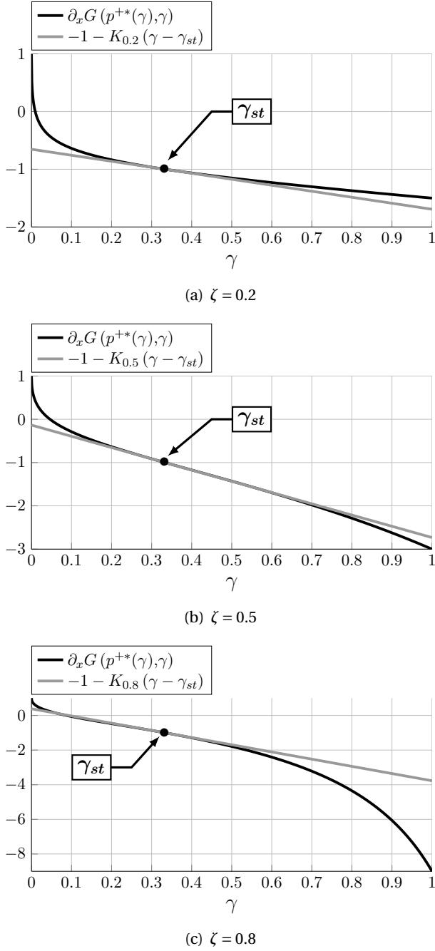
**Figure 3.5 –** Graphical representation of  $\partial_x G(p^{+*}(\gamma), \gamma)$  and its tangent function  $-1 - K(\gamma - \gamma_{st})$  around the static oscillation threshold for  $\zeta = 0.2, 0.5$  and  $0.8$ .
