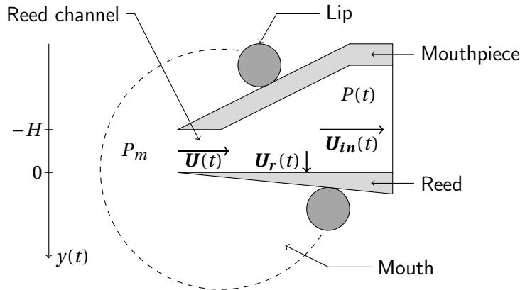
**Figure 2.1 – Schematic diagram of a single-reed mouthpiece.** Presentation of variables, control parameters and choice of axis orientation.  $U$  is the flow created by the pressure imbalance  $P_m - P$  between the mouth and the bore,  $U_r$  is the flow created by the motion of the reed,  $U_{in}$  is the flow entering the instrument,  $y$  represents the position of the tip of the reed and  $H$  is the opening of the reed channel at rest.
