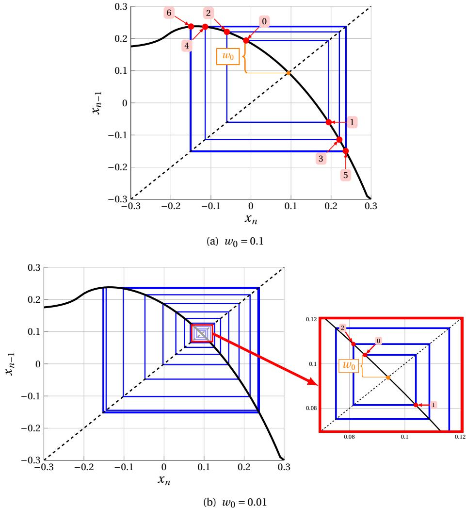
**Figure 4.5** – Graphical solution of equation (4.9) for  $\gamma = 0.42$  and  $\zeta = 0.5$ . (—) Path of the successive iterates 0, 1, 2, etc ; (—) iterative function  $G$  and (- - -) identity  $y = x$ . (a)  $w_0 = 0.1$  and (b)  $w_0 = 0.01$ .
