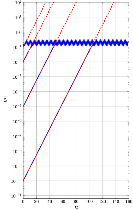
**Figure 4.7** – Graphical representation of the time envelopes of the variable  $w$  using a logarithmic scale for the ordinate axis. (—) envelope obtained from the numerical solution of equation (4.9) and (---) envelopes deduced from the function (4.17).
