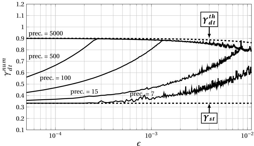
**Figure 2.10** – Graphical representation of  $\gamma_{dt}^{num}$  as a function of  $\epsilon$  for  $\zeta = 0.5$ ,  $\gamma_0 = 0$  and using five different precisions. A logarithmic scale is used in abscissa.
