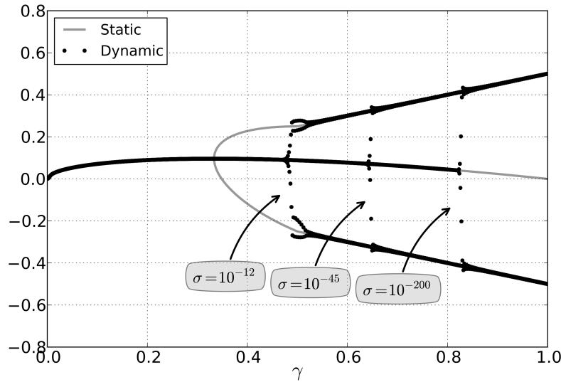
**Figure 4.12** – Static and dynamic bifurcation for  $\zeta = 0.5$ . Dynamic diagram is obtained with  $\epsilon = 10^{-3}$  and  $\gamma_0 = 0$ . Moreover, an ad hoc additive white noise is introduced in system (4.18) with three different levels :  $\sigma = 10^{-12}$ ,  $\sigma = 10^{-45}$  and  $\sigma = 10^{-200}$ .
