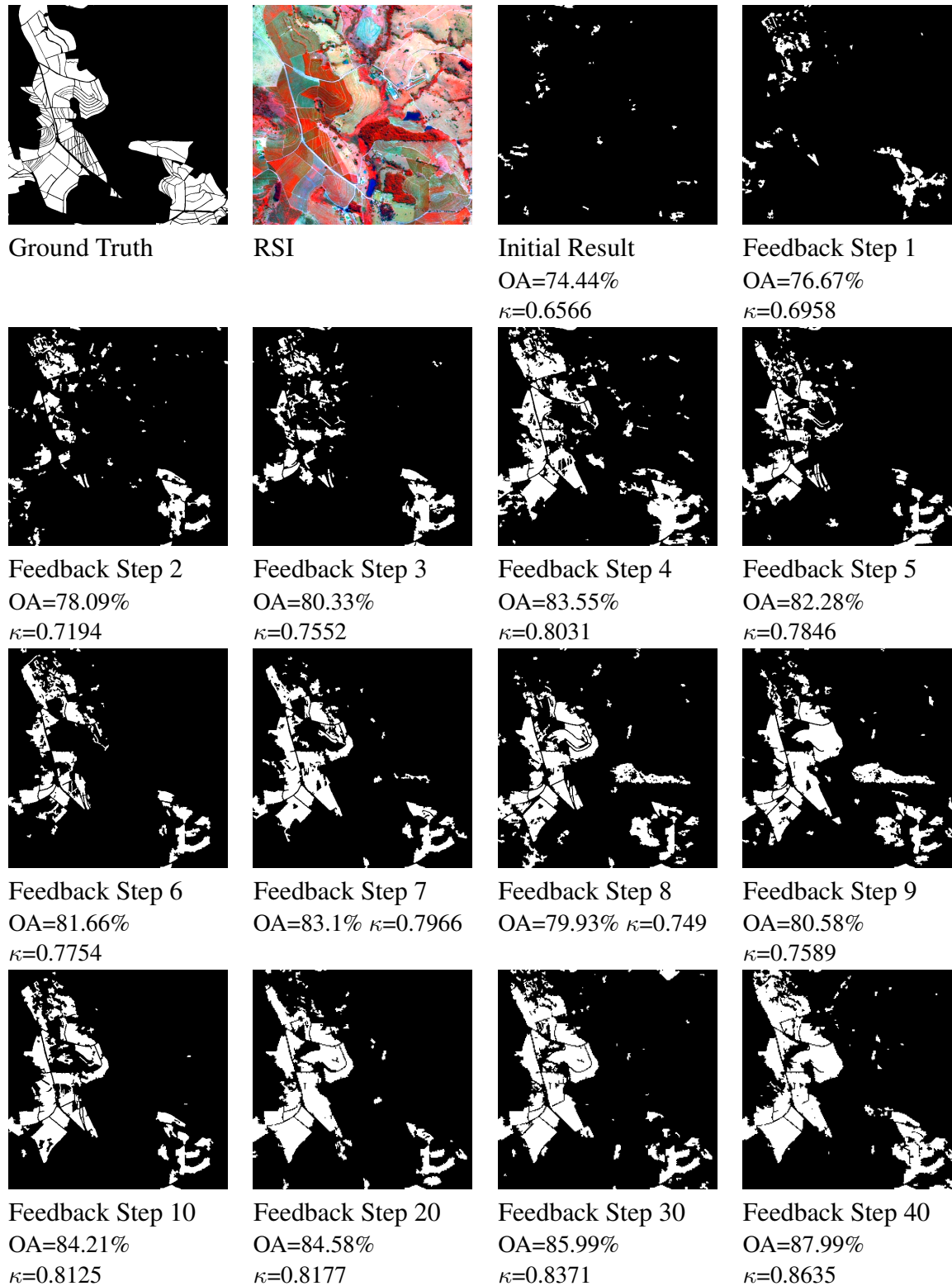
Figure 6.4: Example of the results from the initial classification to the feedback step 10, 20, 30, and 40 compared to the original image and the ground truth. Coffee and non-coffee regions are represented in white and in black respectively. OA=Overall Accuracy; \kappa =Kappa index.
