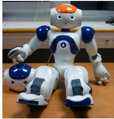
Figure 3.4: Within this work we used a new audio-visual head that is composed of a synchronized camera pair and two microphones. This “orange” head replaces the former “blue” head and is fully interfaced by the RSB middleware previously described in this section.
