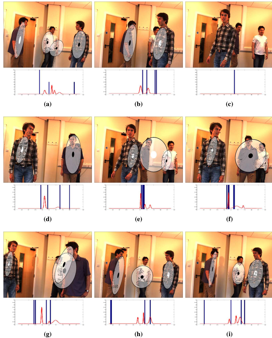
Figure 3.9: Results obtained with the CTMS3 sequence from the CAVA data set. The ellipses correspond to the 3D covariance matrices projected onto the image. The circle at each ellipse center illustrates the auditory activity: speaker emitting a sound (white) or being silent (black) during each time interval. The plot associated with each image shows the auditory observations as well as the fitted 1D mixture model.
