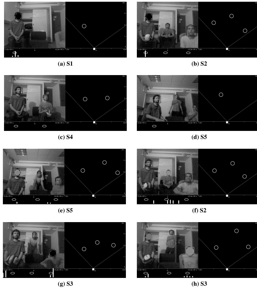
Figure 3.10: Snapshots of the visualization tool. Frames selected among the five scenarios to show the method's strengths and weaknesses. The faces' bounding box are shown superposed to the original image (top-left). The bird-view of the scene is shown in the top-right part of each subimage. The histogram of ITD values as well as the projected faces are shown in the bottom-left. See Section 3.6.3 for how to interpret the images above.
