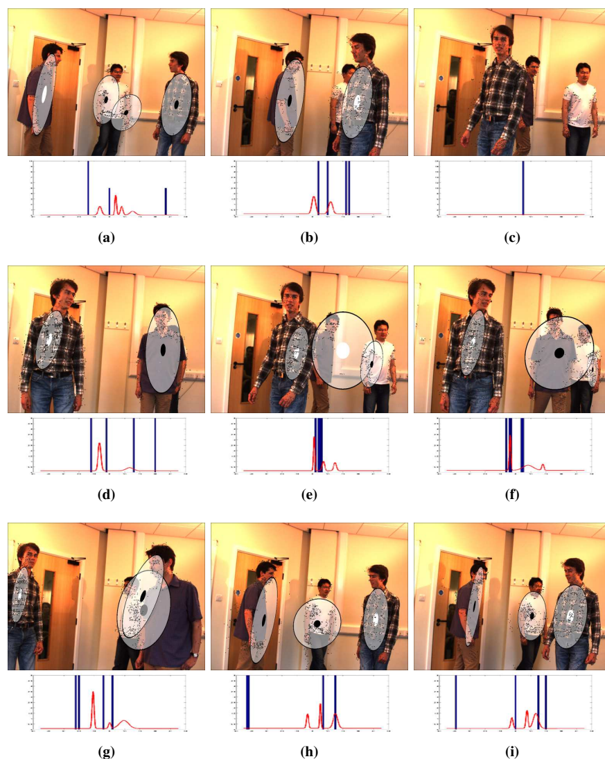
Figure 3.9: Results obtained with the CTMS3 sequence from the CAVA data set. The ellipses correspond to the 3D covariance matrices projected onto the image. The circle at each ellipse center illustrates the auditory activity: speaker emitting a sound (white) or being silent (black) during each time interval. The plot associated with each image shows the auditory observations as well as the fitted 1D mixture model.
