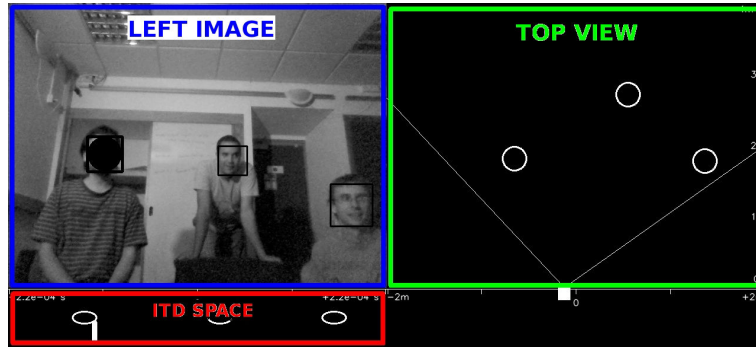
Figure 3.5: Snapshot of the visualization tool. The top-left (blue-framed) image is the original left image plus one bounding box per detected face. In addition, an intensity-coded circle appears when the speaker is active. The darker the colour is, the higher the speaking probability is. The top-right (green-framed) image corresponds to the bird-view of the scene, in which each circle corresponds to a detected head. The bottom-left (red-framed) image represents the ITD space. The projected faces are represented by an ellipse and the histogram of extracted ITD values is plot.
