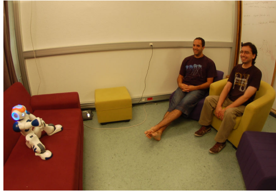
Figure 3.1: A typical scenario in which a companion humanoid robot (NAO) performs audio-visual fusion in an attempt to detect the auditory status of each one of the speakers in the room. The system described processes the raw data gathered with the robot's camera and microphone pairs. The system output is a speaking probability of each one of the actors together with the 3D location of the actors' faces.
