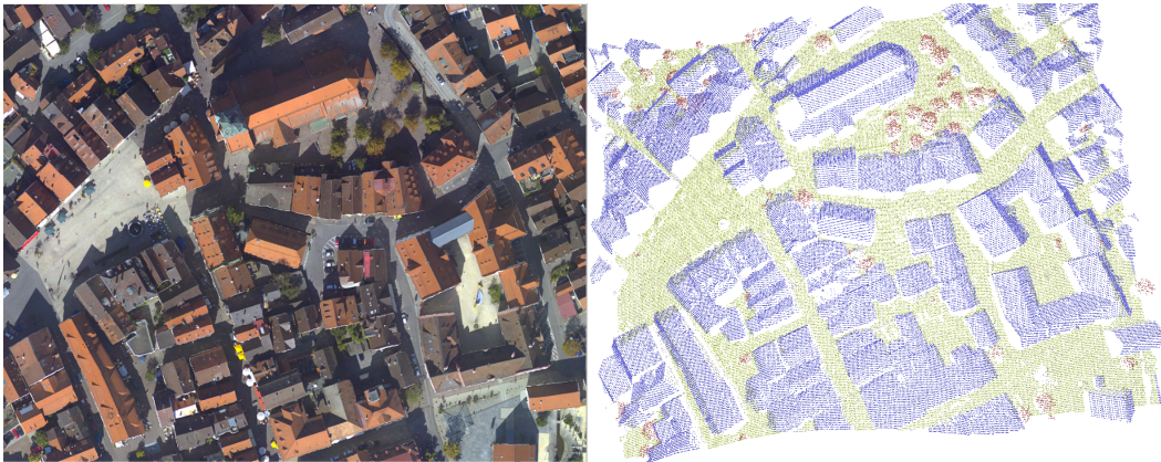
Figure 2.2: Point cloud classification- An aerial image ( left ) and the classified point set ( right ). Note that the four classes building (in blue), vegetation (in red), ground (in green), and NC (in white) are correctly separated.
