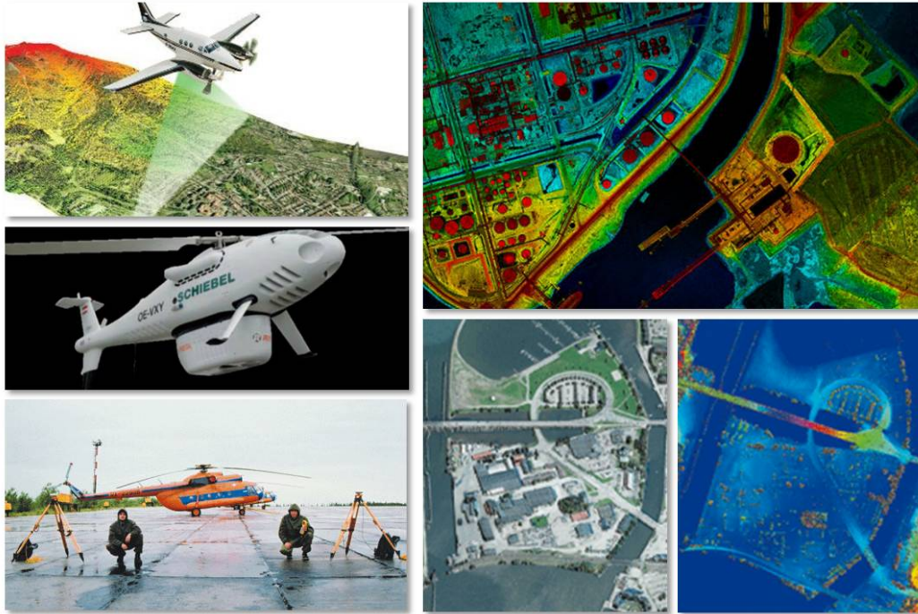
Figure 1.7: Illustration of Airborne Laser Scanner (ALS) and airborne Lidar data. Left column: acquisition vehicle for airborne Lidar measurement. Right column: Airborne Lidar data with color corresponding to the different amplitudes of the backscattered signal. Images courtesy of [Geoinformatics 2007].
